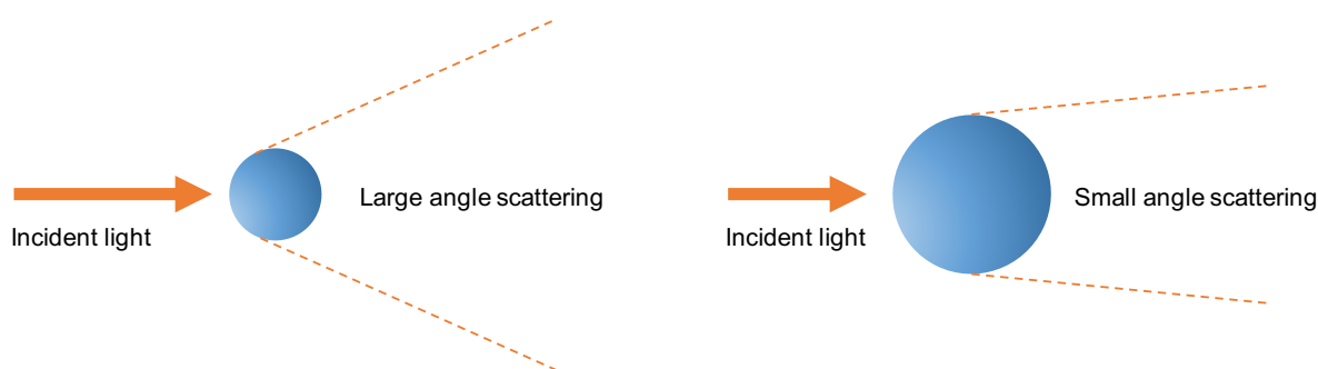
Figure 3.6. Schematic diagram of the incident light source interacting with particles of various sizes.
