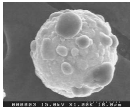
Figure 2.9 - SEM of encapsulated n-pentadecane with a mean diameter of 44 \mu\text{m} (Tseng et al., 2005).
