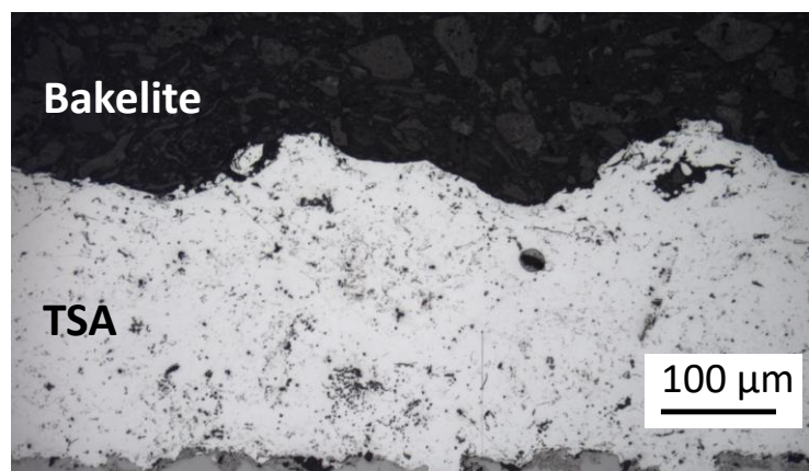
Figure 6-17 Optical micrograph of a cross-section of uncorroded TSA coating showing surface morphology.
