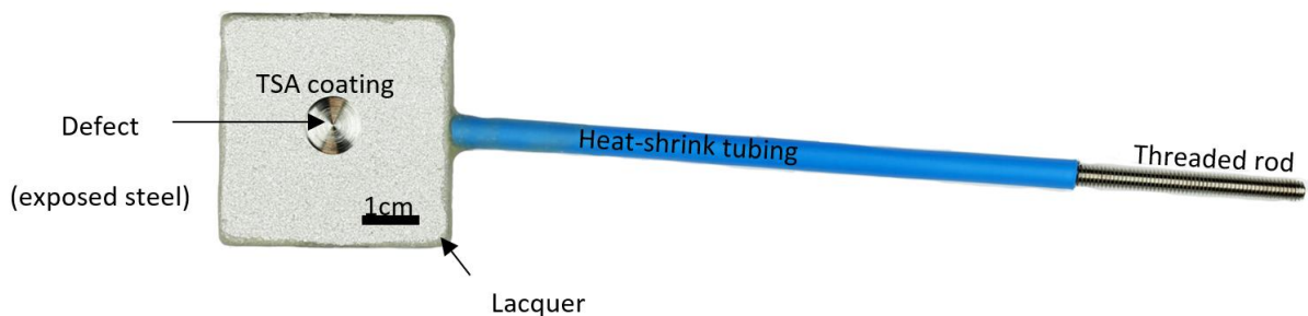
Figure 3-2 TSA-coated steel sample with 5% of the coating area removed to simulate a defect in the coating.
