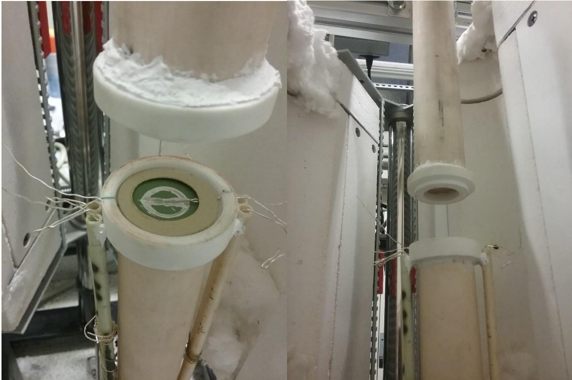
Figure 4-27: Male and female end closure connectors designed to improve leak-tightness.
