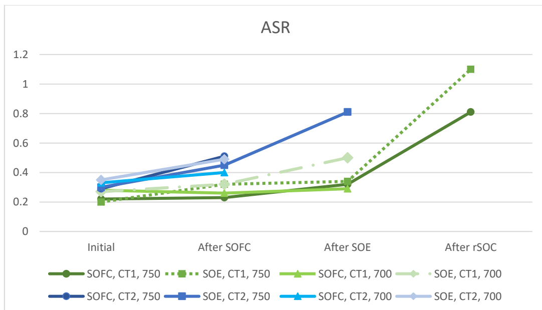
Figure 7-4: ASR comparison of cell types 1 and 2 at 700°C and 750°C (captured under SOFC and SOE conditions)
