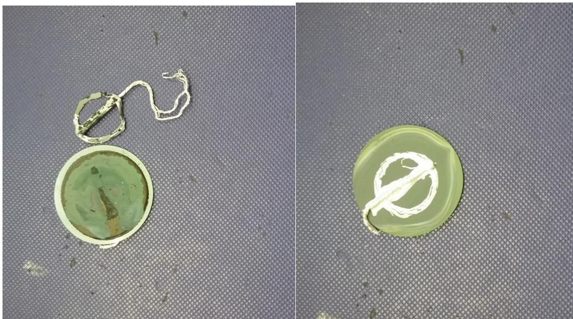
Figure 4-21: Degradation of the silver-based current collectors under test conditions.
