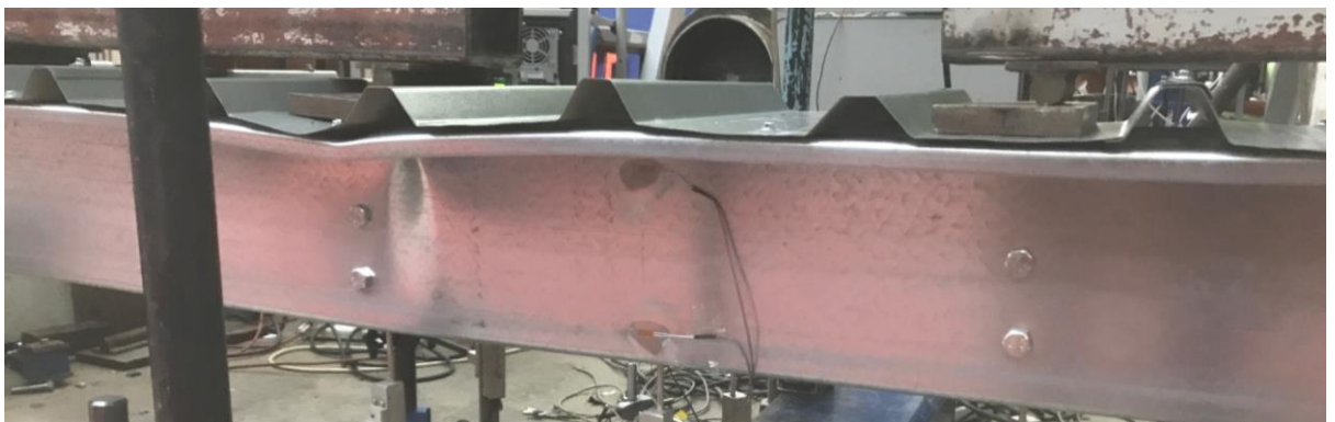
Figure 3.11 Failure mode of Z20620 - distortional buckling and web crippling after the peak load.
