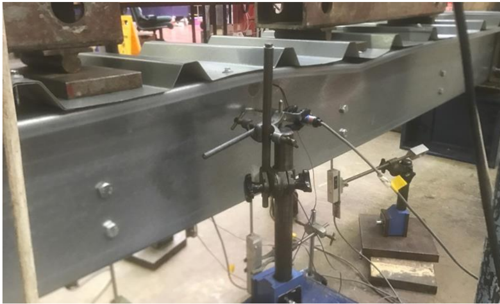
Figure 3.13 Failure mode of Z24620 - distortional buckling.
