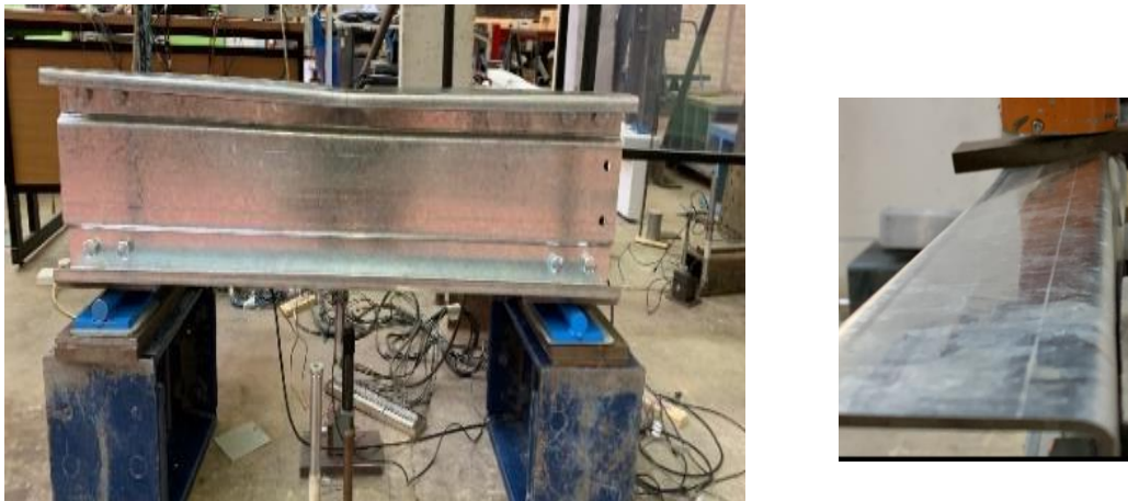
Figure 5.6 Web crippling of the upper web of specimen 26525-50.
