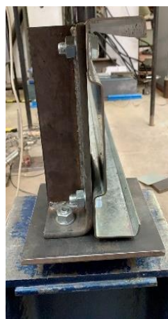
Figure 5.3 Web crippling test set up.
