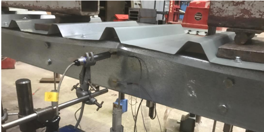
Figure 3.7 Failure mode of Z14613 - interaction of distortional buckling with local buckling of the lip at mid-span.
