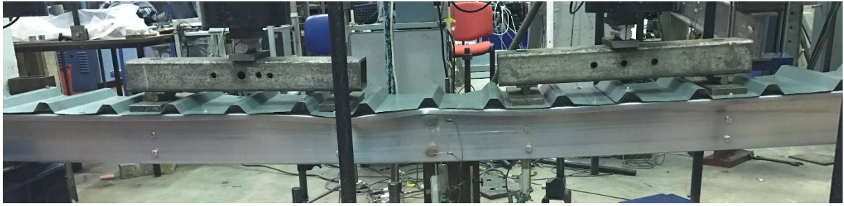
Figure 3.10 Failure mode of Z17625 - distortional buckling and interaction with local buckling of lip following material yielding.
