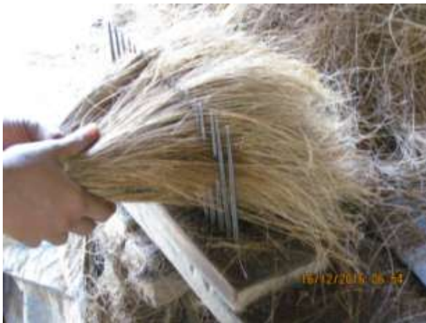
Figure 4.11 photograph of coir fibres showing the combing of coir fibres after dehusking (Courtesy of G. Fernando, University of Birmingham).
