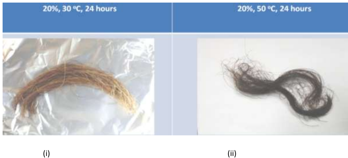
Figure 4.36 Photographs of NaOH-treated fibres showing change in colour at (i) 20% NaOH concentration, 30 °C and for 24 hours duration and (ii) 20% NaOH concentration, 50 °C and for 24 hours duration
