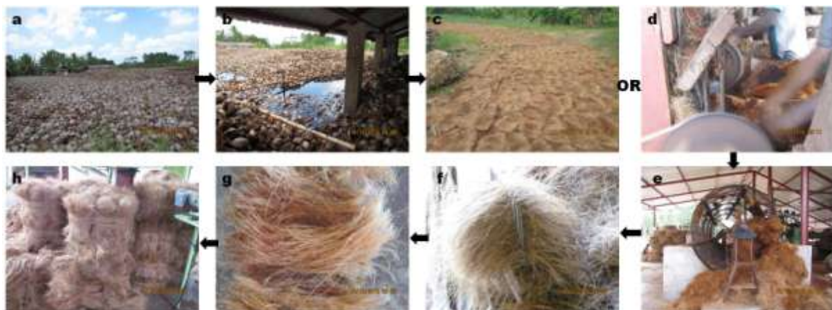
Figure 2.13 Basic processes of production of coir fibre [courtesy: G Fernando, University of Birmingham].
