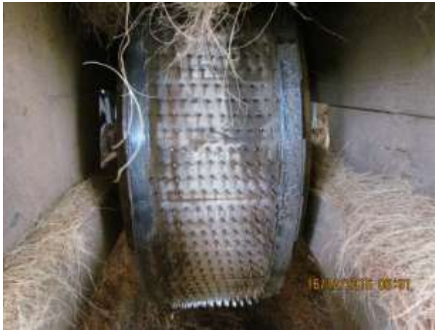
Figure 4.8 A photograph of the drum with spikes used to separate coir fibres from the husk (Courtesy of G. Fernando, University of Birmingham).
