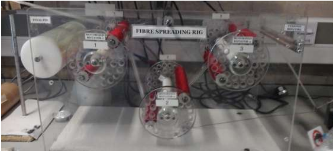
Figure 3.10 Key components of the fibre spreading rig.
