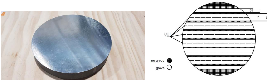
Figure 3.1: Inconel 718 substrate before machining and the top view layout for the machining process (all is in mm)
