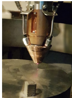
Figure 3.4: The three-beam nozzle used in the experiment
