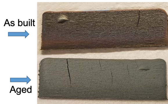
Figure 7.10: Failed samples that cracked during deposition, before and after heat treatment
