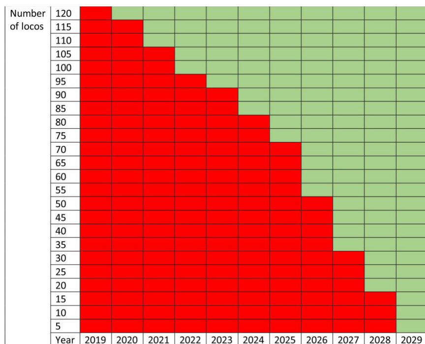
Diagram 6-09 Red squares indicate number of locomotives in service in each year with a current boiler certificate. Green indicates the minimum number of locomotives required to complete their ten-year overhaul to keep the total number of locomotives constant. Number refer to ex BR locomotives. This shows that fewer locomotives are required to be overhauled than were completed over the last ten years, thus if the same level of activity is undertaken, sustainability of the fleet can be maintained.
