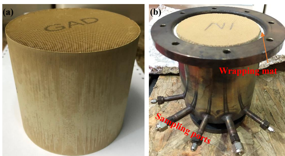
Figure 3-7. (a) TWC monolith (b) TWC fitted into the aftertreatment canning
