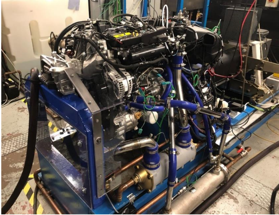
Figure 3-2. The three-cylinder DI/PFI gasoline engine testing bench
