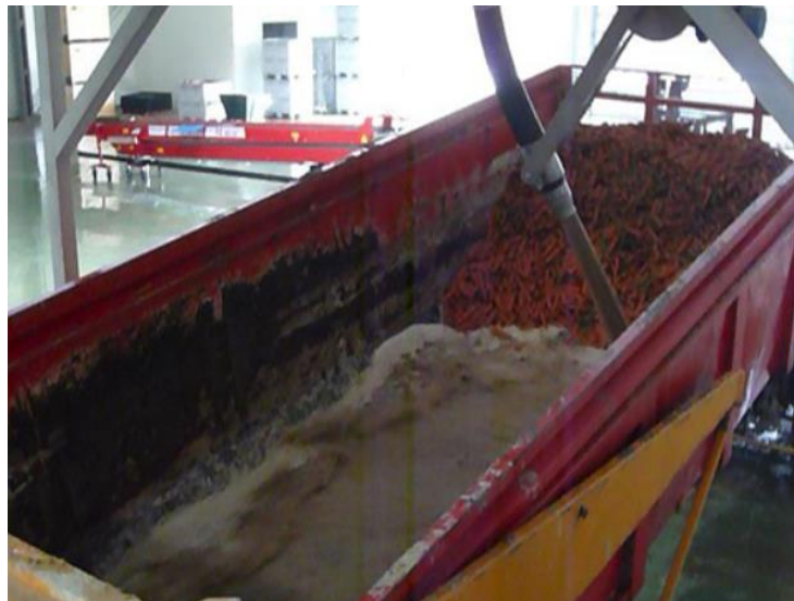
Figure 3.1.2.1) Image by Haith Ltd. (2020) illustrating unloading roots (carrots in this case) from transport trailer via use of gravity and overhead water pipes.
