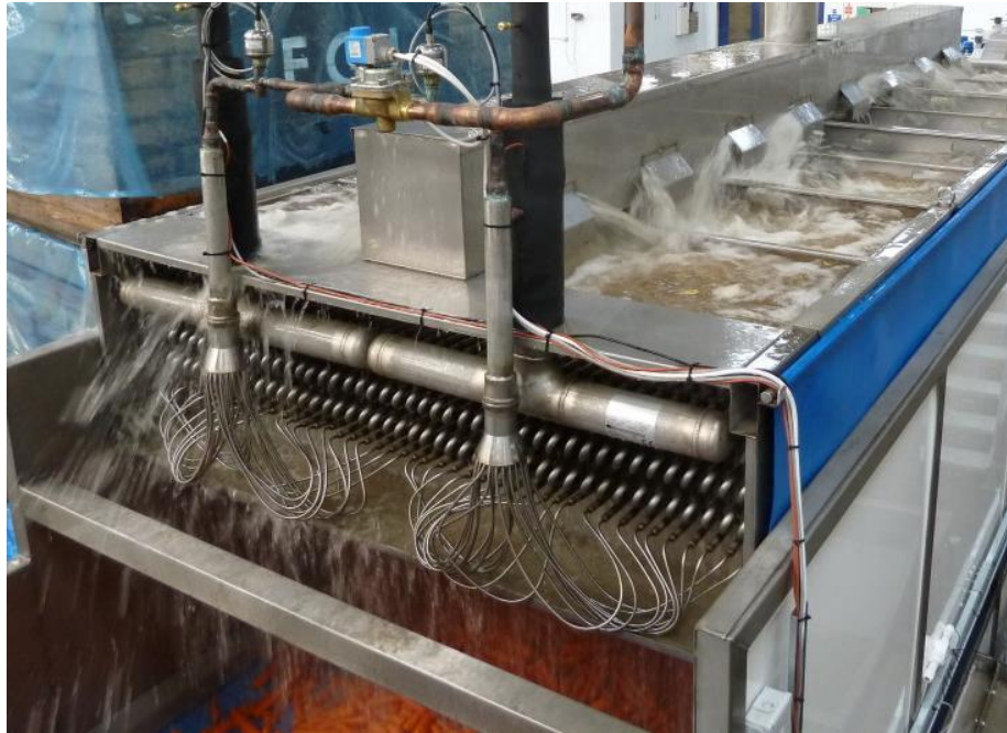
Figure 3.1.6.0) Image by Haith Ltd (2020) showing root hydrocooler reducing the temperature of carrot roots before they enter cold storage.
