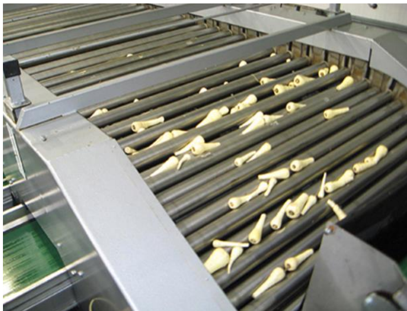
Figure 3.1.5.0) Image by Haith Ltd, (2020) illustrating grading of parsnip roots by crown diameter (mm) in a UK parsnip packhouse.
