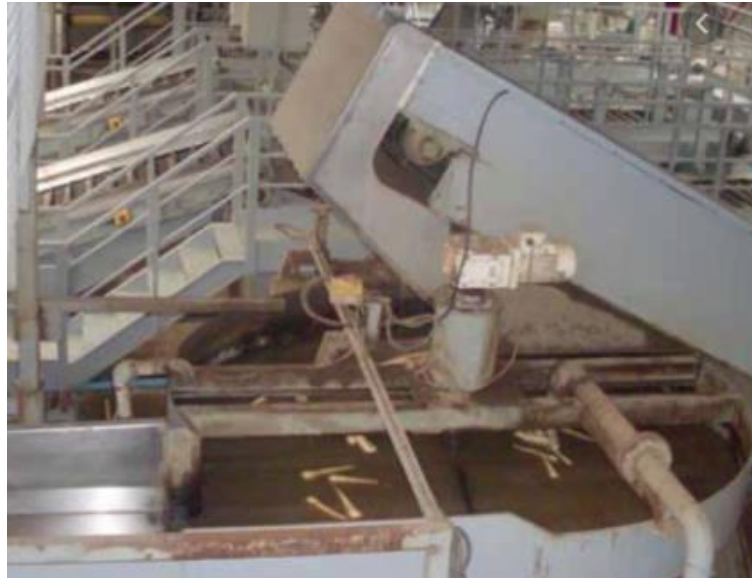
Figure 3.1.2.2) Image by tnicltd UK, 2020 illustrating parsnip roots being cleaned in a cyclone destoner following unloading from transport and intake into the packhouse.
