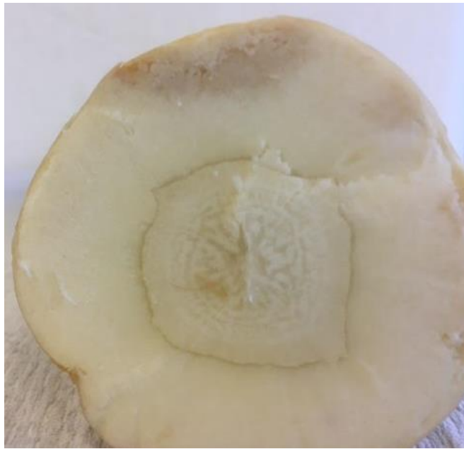
Figure 1.3.2) Author's own image demonstrating the development of bruising damage in V2 tissue following mechanical impact via falling bolt method, following 48 hours of storage at 20 °C.
