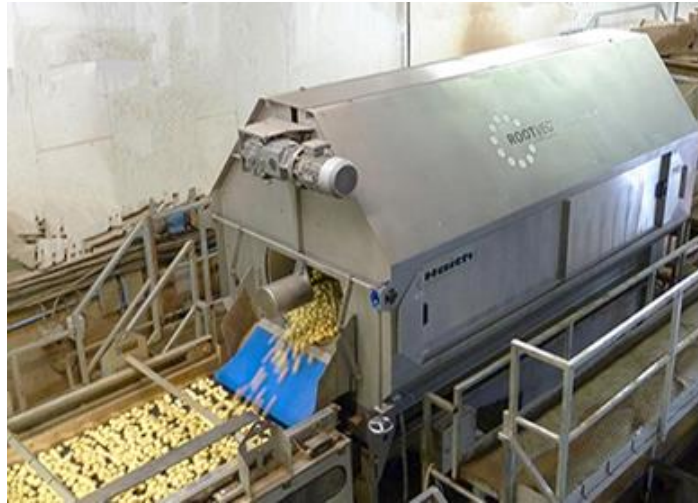
Figure 3.1.4.1) Image by Haith Ltd 2020 illustrating empty root vegetable polisher with independently moving brushes lining the inside of the rotating drum . Not shown is exit door which facilitates users to increase or decrease the period of time roots spend in the polisher and therefore the flow of roots out of the polisher.
