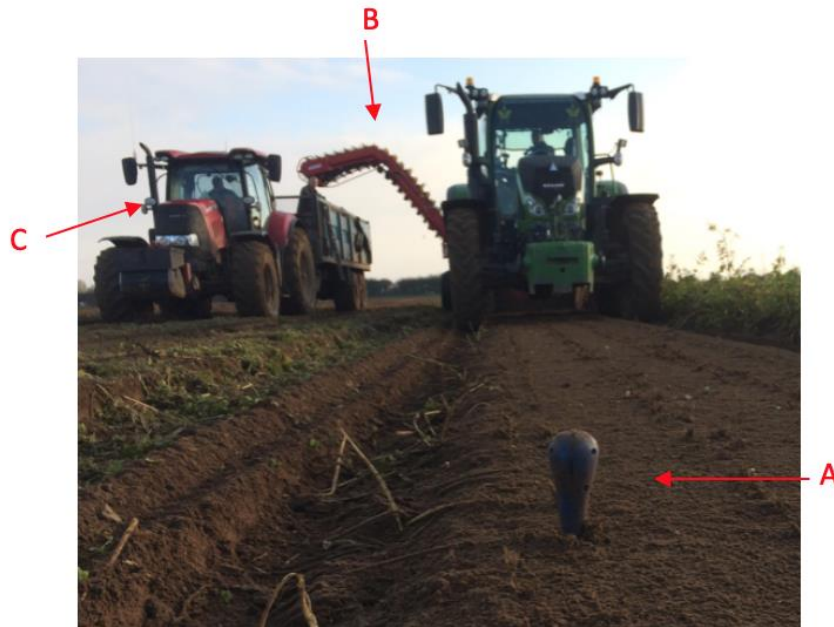
Figure 3.1.1.0) Authors own image illustrating electronic parsnip device (A) inserted into freshly topped row of parsnips. Also shown is loading elevator chute (B) and loading trailer (C).
