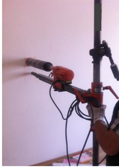
a) Core sample taking for concrete quality control
