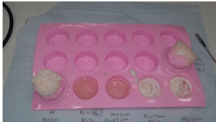
Figure 78. TCM/PCM-gel preparation after drying in the humidity chamber at 70 °C
