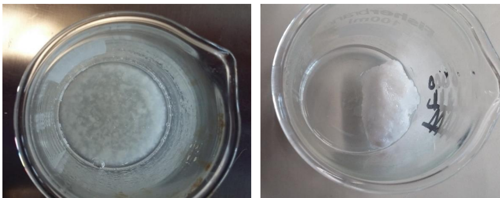
Figure 63. Left; Mixture of Gel and TCM with an order of addition 1 st TCM and 2 nd gel following the procedure described in the methodology section. Right; Mixture of Gel and TCM with an order of addition 1 st gel and 2 nd TCM following the procedure described in the methodology section.
