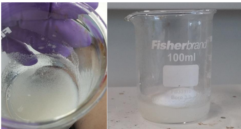
Figure 66. Right: phase segregation; Left: lumps heterogeneously distributed.
