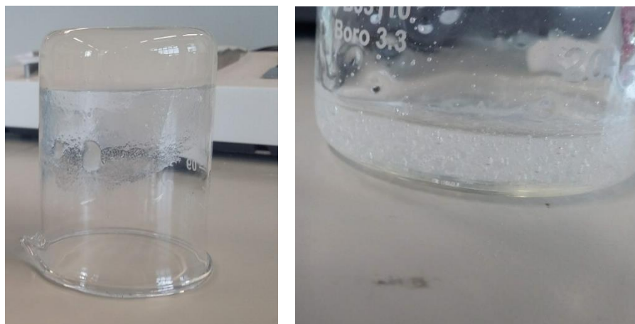
Figure 63. Left; Mixture of Gel and TCM with an order of addition 1 st TCM and 2 nd gel following the procedure described in the methodology section. Right; Mixture of Gel and TCM with an order of addition 1 st gel and 2 nd TCM following the procedure described in the methodology section.
