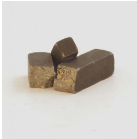
Figure 4.8: Terfenol-D rods are typically formed in cylindrical or bar shaped geometries. 119 Attention should be drawn to the brittle fracture surface which is indicative of both the catastrophic failure mode and limitations of Terfenol-D.
