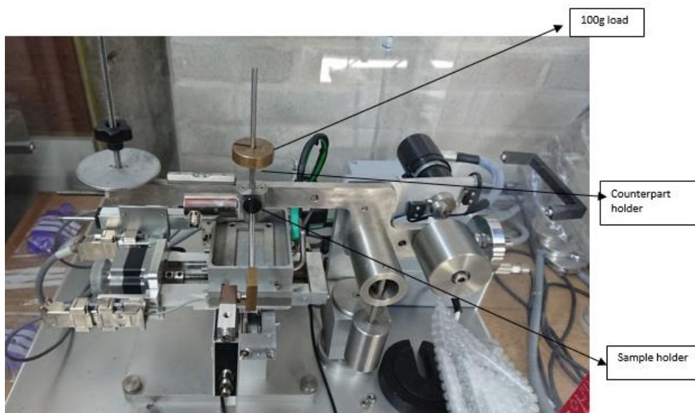
Figure 3.5.1b. Image depicting the set-up for the wear tests.
