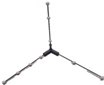
Figure 73 Wand and axes for calibration of equipment prior to OEP recording
