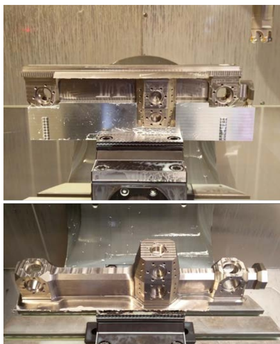
Figure B.1: Photographs of the machining of the vacuum chamber.
