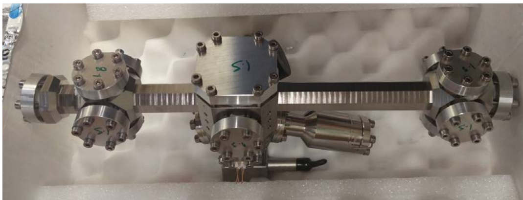
Figure B.5: Photographs of the vacuum system with the Indium seals on and ready for vacuum preparation.
