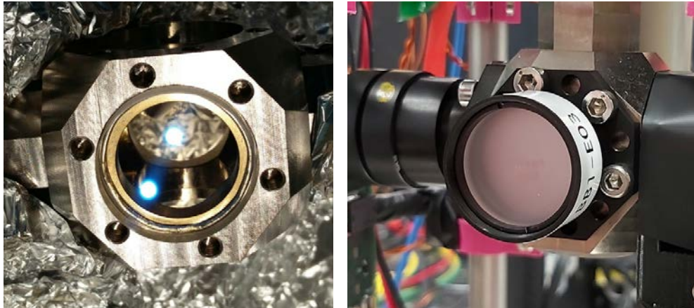
(a) Photograph of a completed window. (b) Photograph of the window adaptor with mirror.
