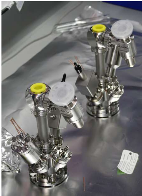
Figure 3.4 Flange multiplexers from Kimball Physics join vacuum peripheries to science chambers. The two pieces are linked with a flexible and rigid nipple (not shown).
