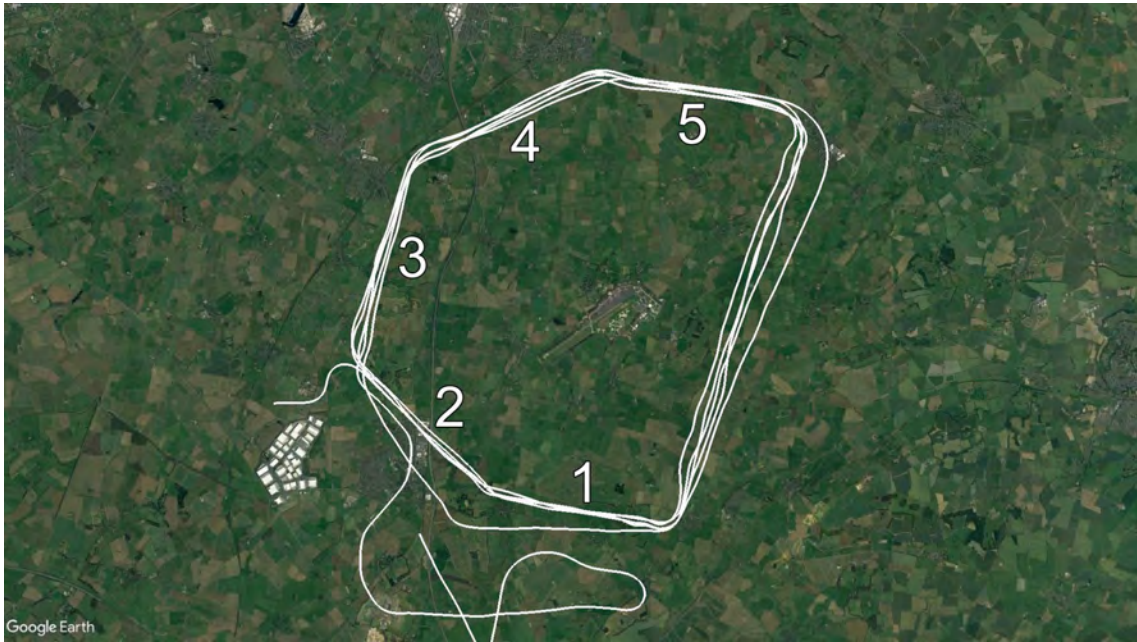
Figure 5.5: Actual flight route of the airborne platform as measured by the GNSS receiver. The different flight segments are labelled from 1-5
