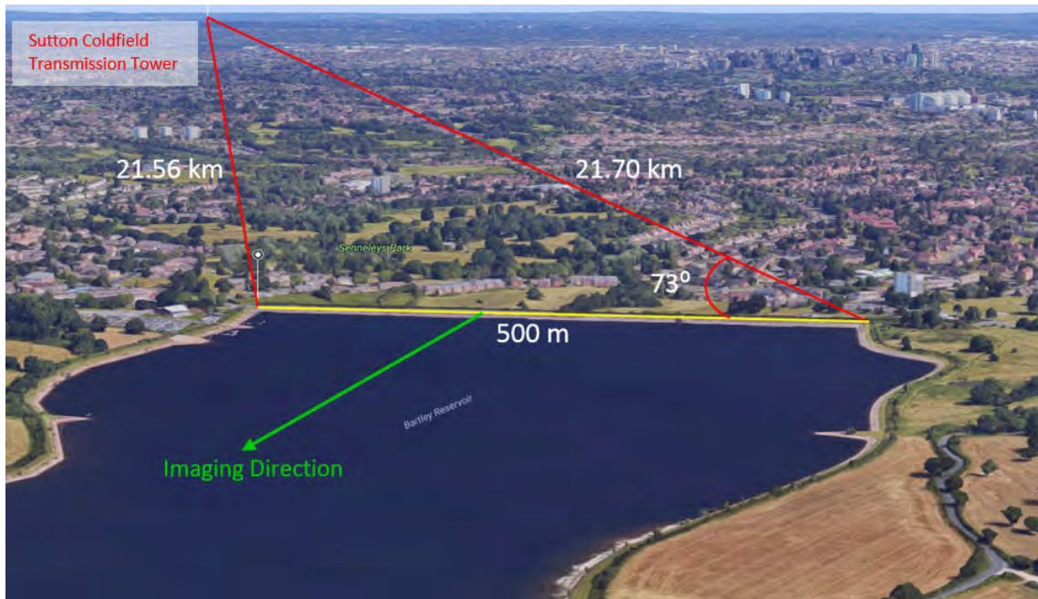
Figure 3.13: Image showing the synthetic aperture relative to the transmitter and Bartley Reservoir
