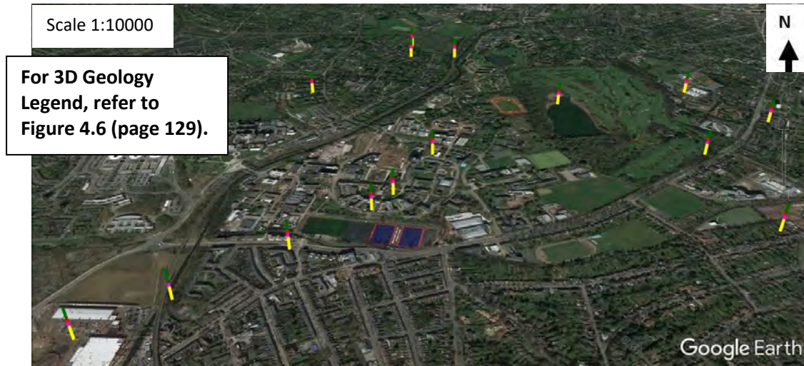
Figure A.5: An integrated visualisation using Google Earth (Google Inc., 2018), showing the borehole locations (cylinders) including their logs.
