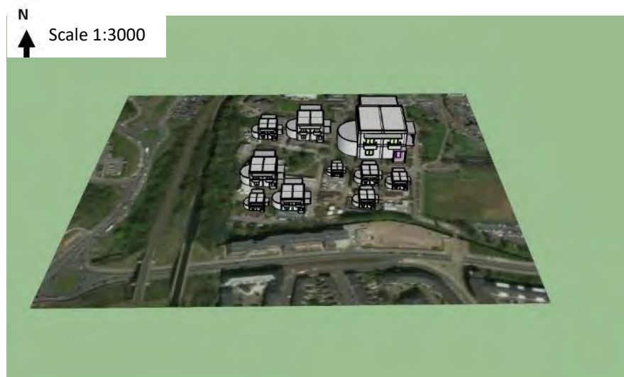
Figure 3.7: Buildings on their georeferenced position in actual topography using BIM (SketchUp) after Providakis et al. (2019).
