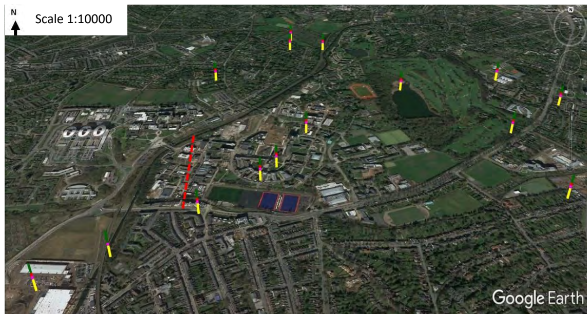
Figure 5.2: The borehole locations around the University of Birmingham, UK, utilised in the modelling demonstrated on Google Earth (Google Inc., 2018). The adopted tunnel is marked with a red dotted line.
