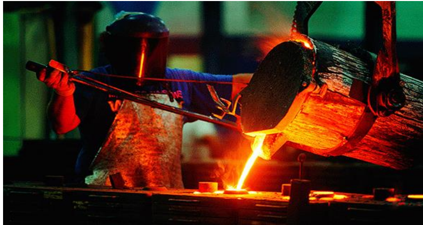
Figure 2-3. Worker pouring molten steel in cast [45].
