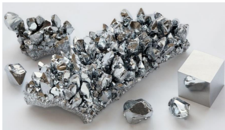
Figure 2-2. Raw chromium crystals (left) and fabricated cube (right) [44].
