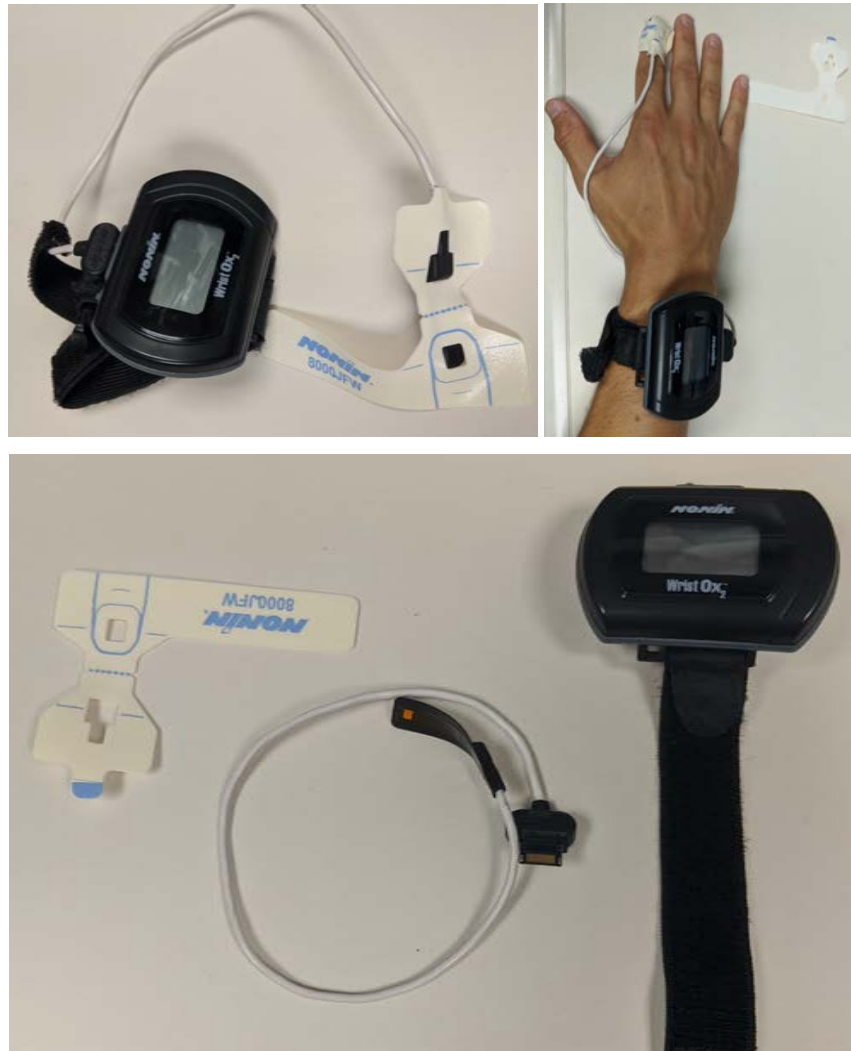
Image 7.1a - c - Portable pulse oximeters and finger sensors. WristOx 3150 Model finger pulse oximeter and 8000J adult flexible finger wrap with disposable adhesive sticker (Nonin Medical). Photo credit to Dr Courtney Wheatley and Mr Jesse Schwarz of the Johnson Lab, Mayo Clinic, Scottsdale campus, Scottsdale, Arizona.
