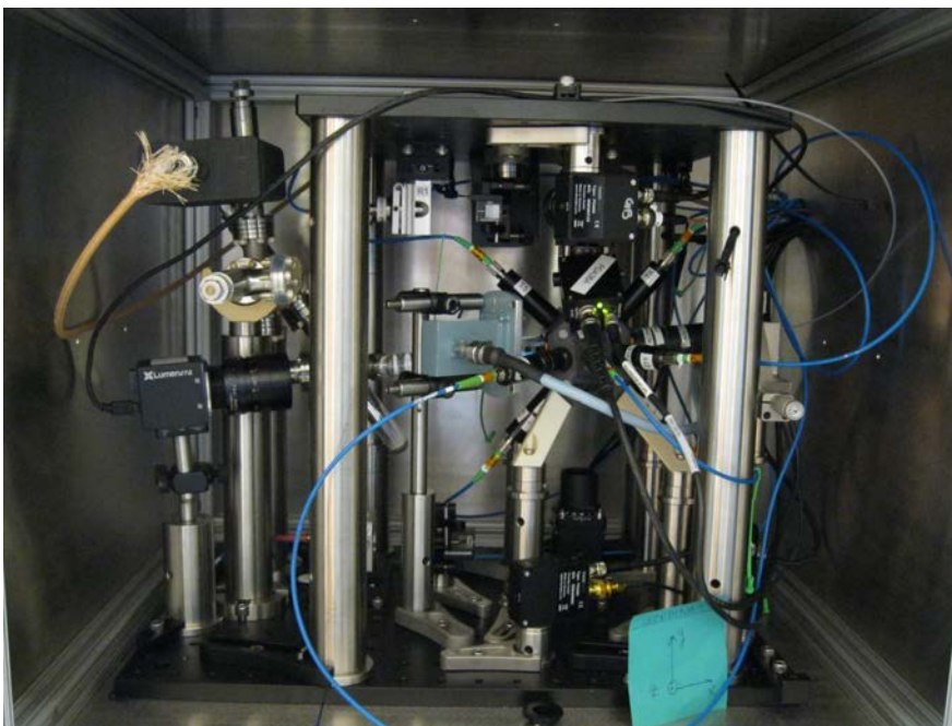
Figure C.1: This photo shows the entire sensor head inside its magnetic shield.
