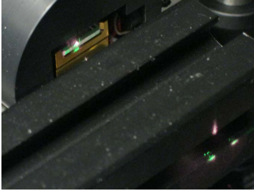
Figure D.1: The green spots are caused by 4-wave mixing within the PPLN doubling crystal, they are visible on the crystal output facet (top left) and on the beam block after a back reflection from the collimating lenses.
