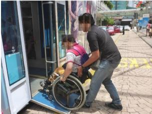
Figure 5-20 Example of accessible bus with manual flip out ramp (a) accessible Smart Selangor bus (b) accessible hop-on-hop-off bus
