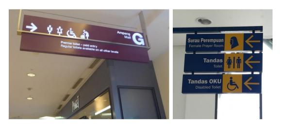
Figure 6-23 Examples of signage to indicate toilet for OKU
