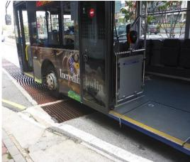
Figure 5-22 Low floor bus (a) no other steps as barrier as OKU entered the bus (b) the ramp is folded in when not in use
