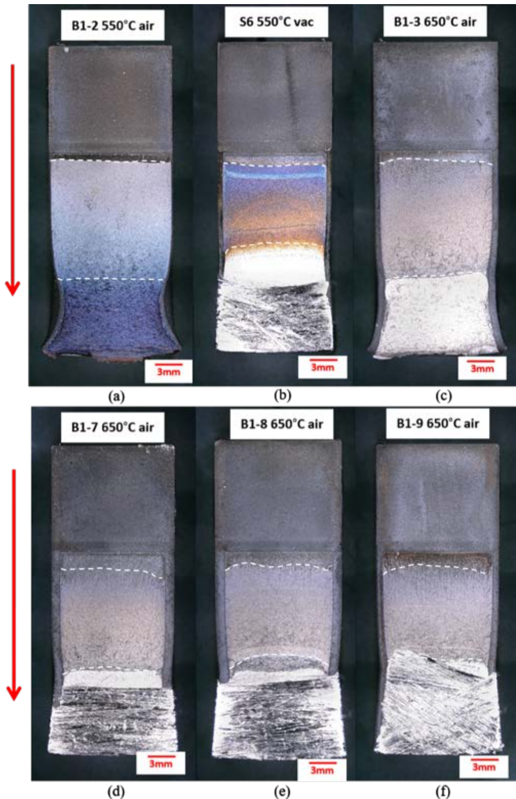
Figure 4.25 Optical fractographs for fatigue crack growth testpieces of the as-received Alloy 709 tested in air at (a), (b) 550, (c) - (f) 650°C, (g) 650°C in vacuum (h) 750°C in air and (i) 750°C in vacuum. Note: Red arrows indicate the direction of crack growth. A back-face notch was applied using a hand saw to facilitate the breaking open of the testpieces. Continued overleaf.
