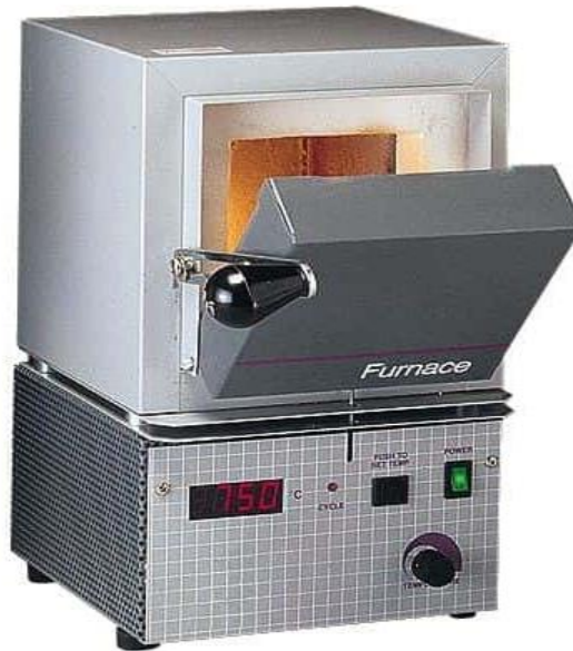
Figure 11 Furnace used for oxidising porous silicon samples.
