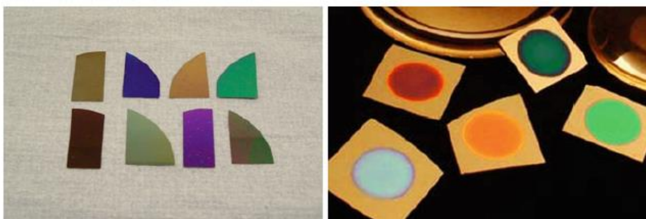
Figure 6 Varied “physical colours” from ultrathin single layers of stain-etched mesoporous silicon (LHS-A. Loni unpublished 2009) and anodised mesoporous silicon photonic crystals (RHS-Gooding Group, Univ. New South Wales, Australia http://www.rsc.org/Publishing/ChemTech/Volume/2009/02/biosensors.asp )
