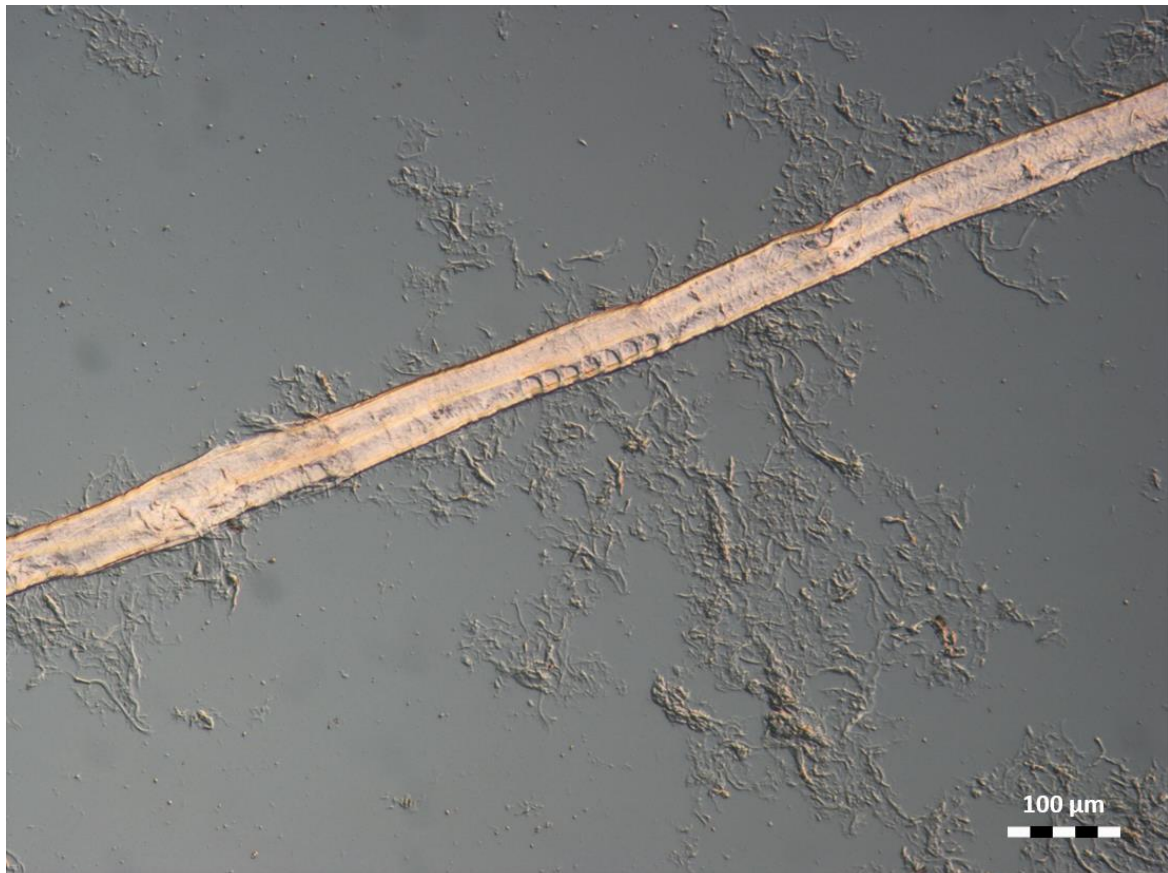
Figure A3.13 – DIC Microscopy Image of 100 POP MFC produced with Glass A media ( R_a = 0.12 \mu\text{m} ) at 12000 kWh/t, showing that some fibres resist breakage, skewing L_c(l) values to higher than they would otherwise be. It is not clear if this is due to the existence of dead zones in the grinder, or if the toughest fibres are able to completely resist grinding from such smooth media.
