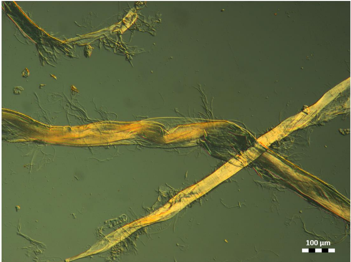
Figure 6.15 – DIC microscopy image of MFC produced at 3000 kWh/t with 2.9 mm media and 300 rpm impeller speed.
