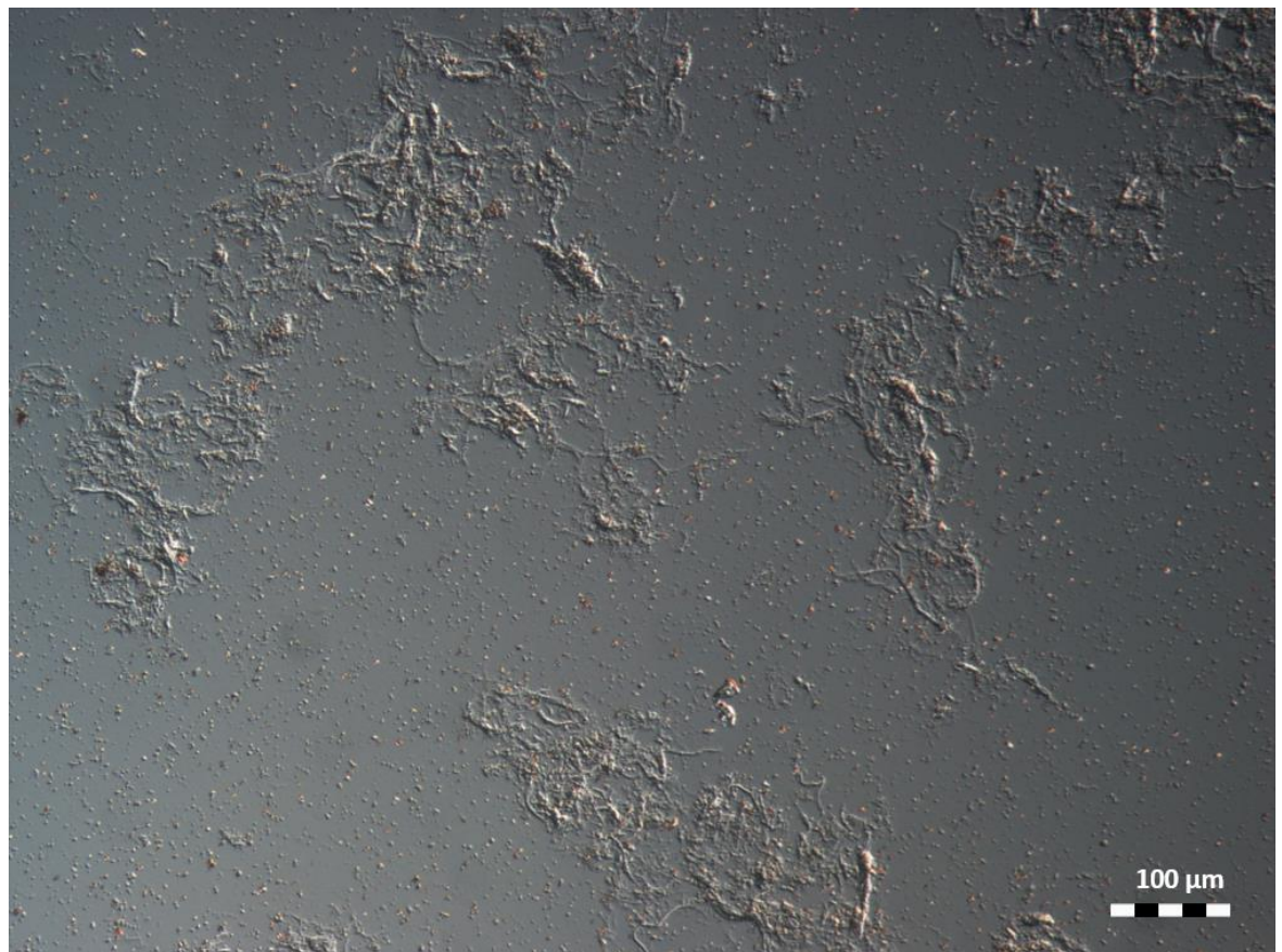
Figure 4.6 – DIC microscopy image of MFC at an energy input of 5000 kWh/t.
