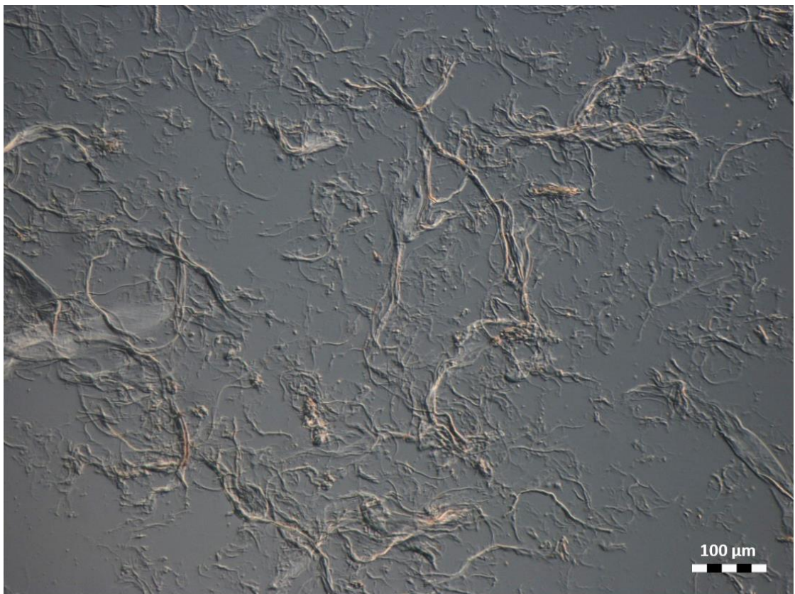
Figure 5.14 – DIC microscopy image of MFC produced at 3000 kWh/t using rough glass (Glass E), R_a = 0.88 \mu\text{m} .
