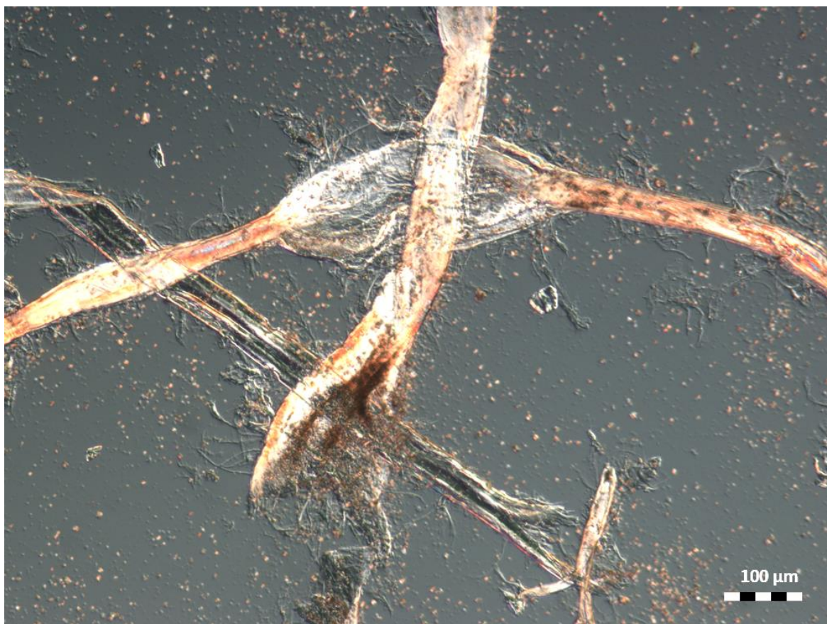
Figure 4.2 – DIC microscopy image of MFC at an energy input of 500 kWh/t.
