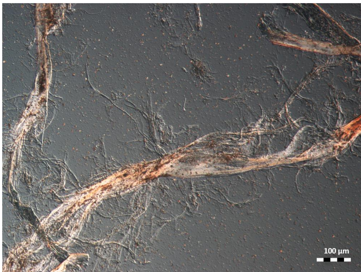
Figure 4.3 – DIC microscopy image of MFC at an energy input of 1000 kWh/t.
