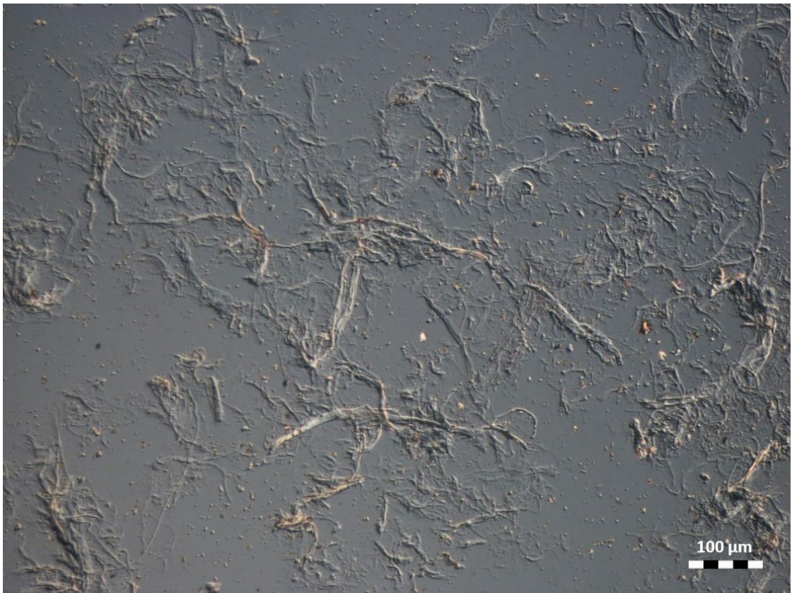
Figure 5.16 – DIC microscopy image of MFC produced at 3000 kWh/t using rough glass (Glass B), R_a = 1.90 \mu\text{m} .
