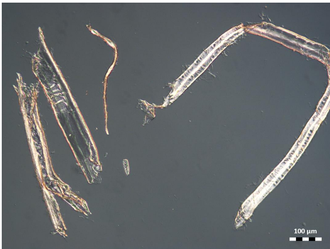
Figure 4.19 – DIC microscopy image of MFC ground to 500 kWh/t in a hygroscopic LiCl solution.
