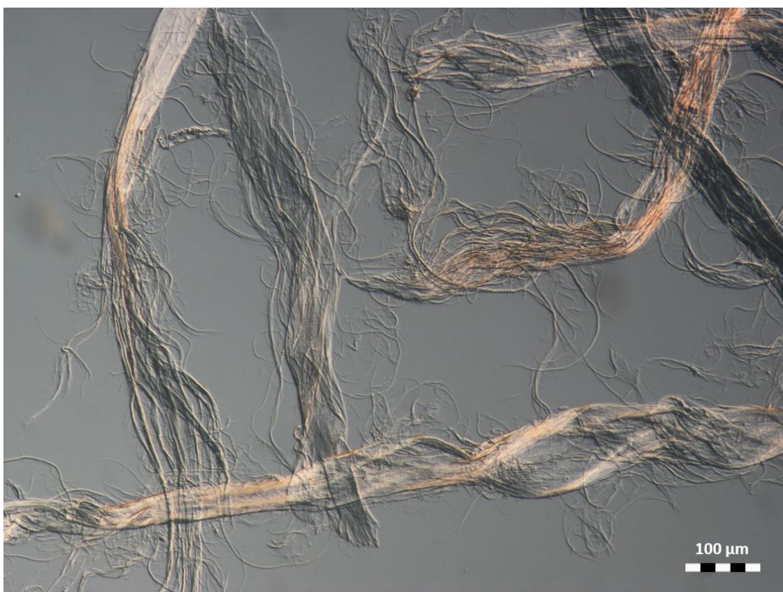
Figure 4.20 – DIC microscopy image of MFC ground to 3000 kWh/t with nylon media, with partially intact fibres.
