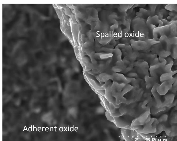
Figure 4.119 – SEI SEM micrographs of oxide formed on Super 304H after oxidation in deoxygenated steam for 100 hours at 650 °C.
