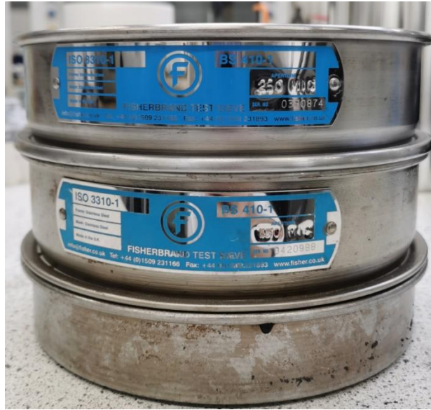
Figure 38 Example of the sieving set up for material preparation of EG.
