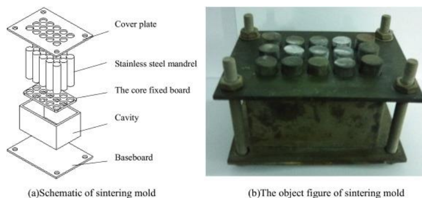
Figure 30 Schematic of the sintering mould [164].
