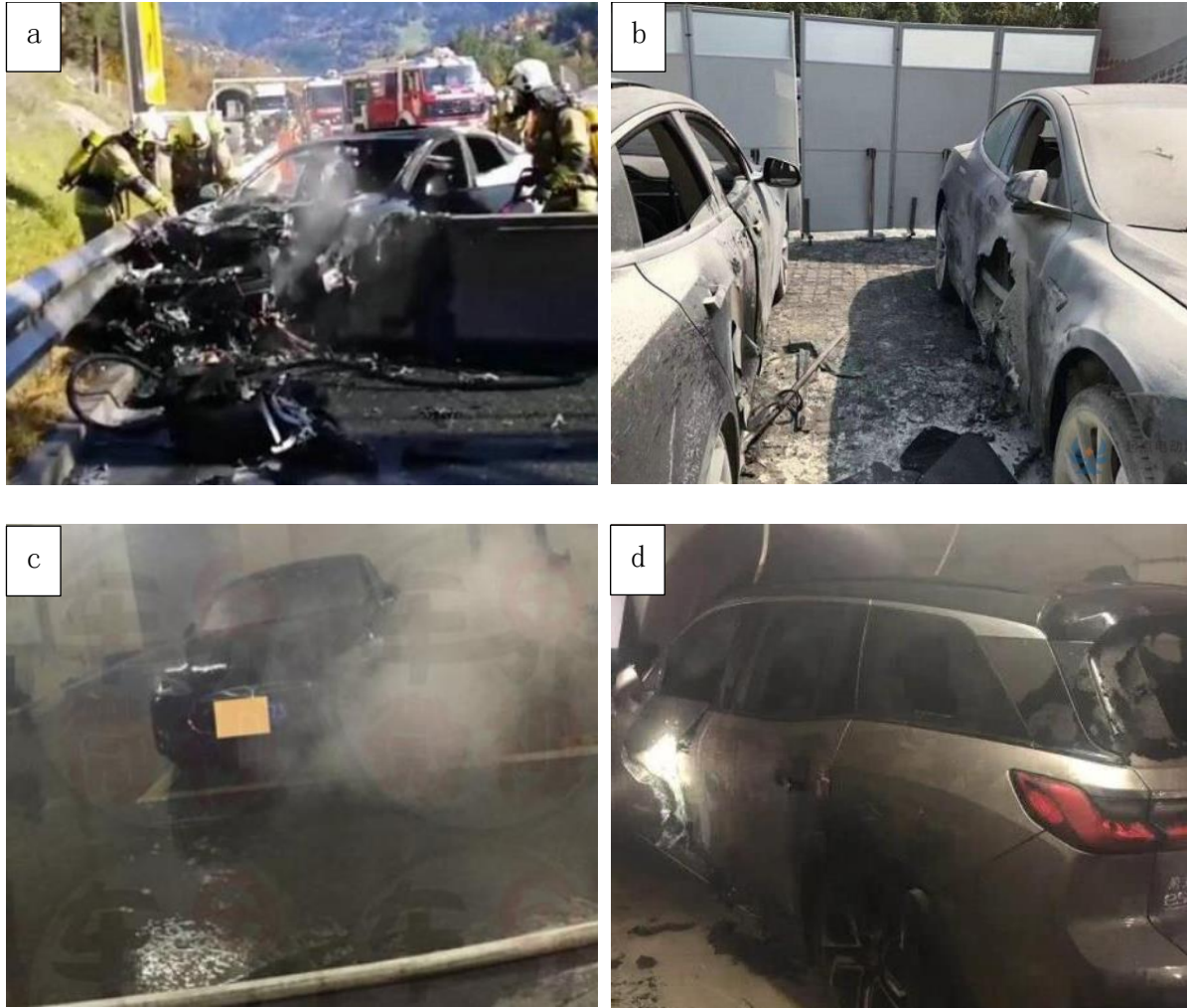
Figure 14 (a) Austria (2017) Tesla Model S, battery short circuit due to the force deformation of the chassis in a collision, [123]; (b) Shanghai, China (2017) two Tesla Model S caught fire at a charging station [123]; (c) Chongqing, China (2018) Tesla Model S spontaneously ignites due to battery failure [125]; (d) Shanghai, China (2020), NIO ES8 caught fire at charging station [117]
