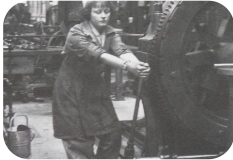
5. A girl operates a rifling machine at the Gun Factory, Royal Arsenal, Woolwich.
