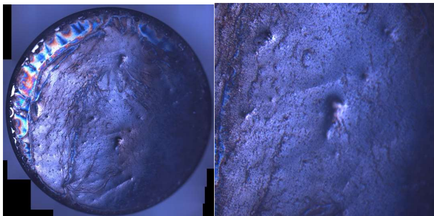
Figure A7.1- 42 \mu\text{L} of 1 to 10^{-4} DNA-cisPt hot plate 255^\circ\text{C} , 30 minutes.
