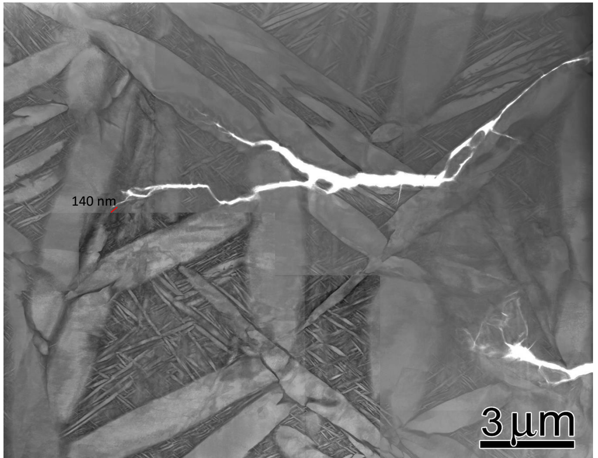
Figure 9.21: Measurements taken of the oxide length ahead of the crack tip for the air test at 500°C.
