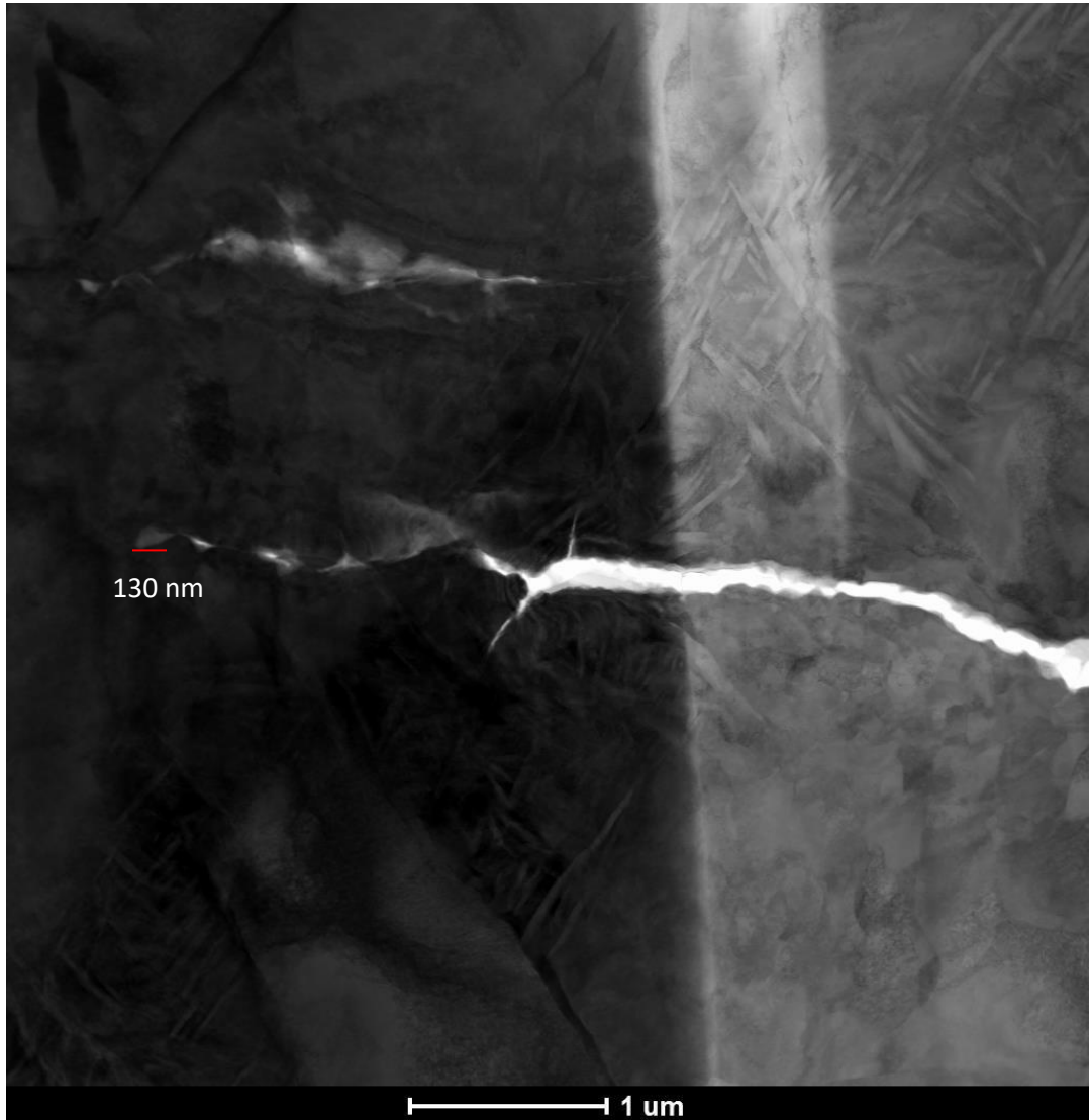
Figure 9.22: Measurements taken of the oxide length ahead of the crack tip for the vacuum test at 500°C.
