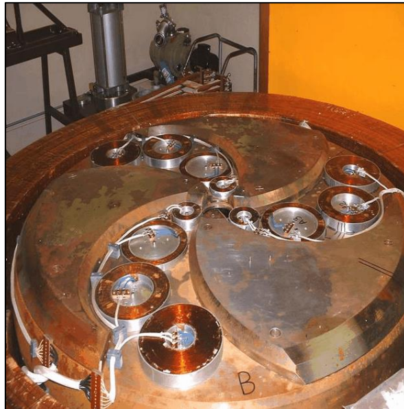
(Figure 5: Magnet Face Showing Spiral Hill / Valleys and Additional Beam Focusing Magnets (Nuclear Physics Research Group, 2012)).
