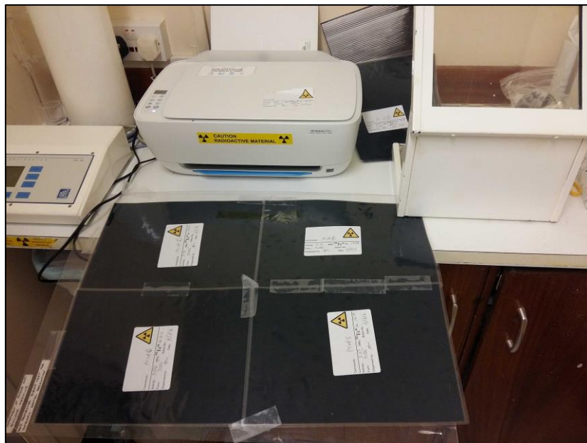
(Figure 21: Photo Showing Composite Flood Source in Foreground, with Inkjet Printer Behind. Image taken at City Hospital Birmingham, Hot Lab).
