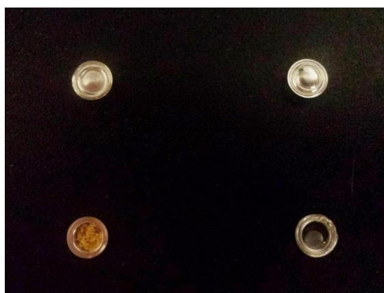
Figure 5-7: Silymarin DSC pans pre (left) and post (right) heating (sealed (top) and uncovered (bottom) views).
