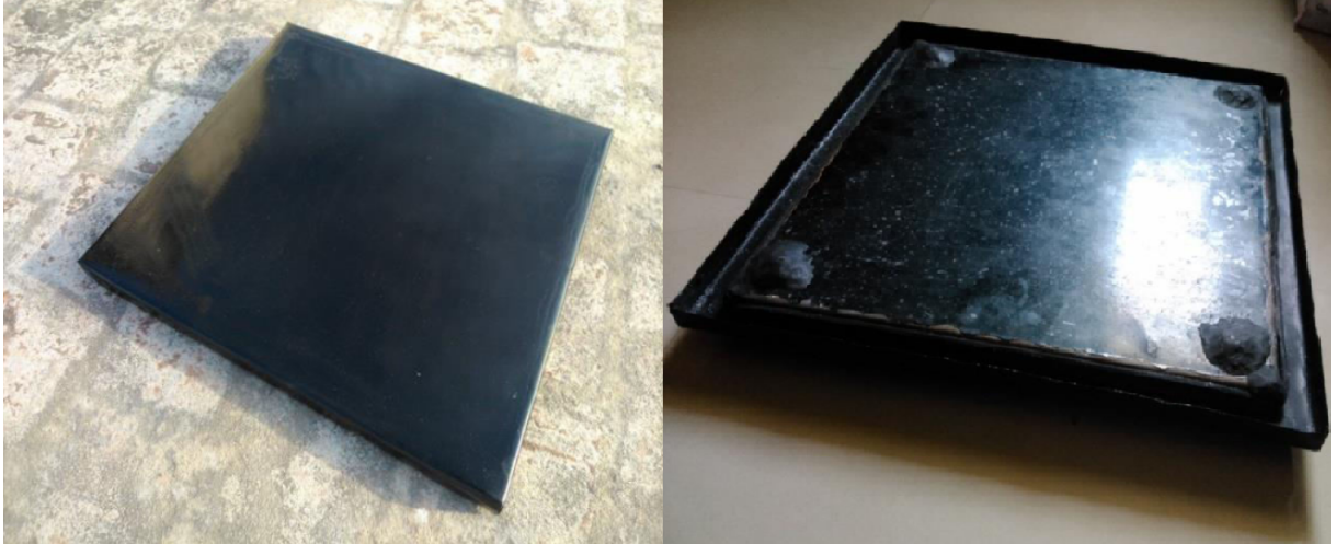
Figure 2.12: The comparison image of vehicle ceiling without/with PCM
