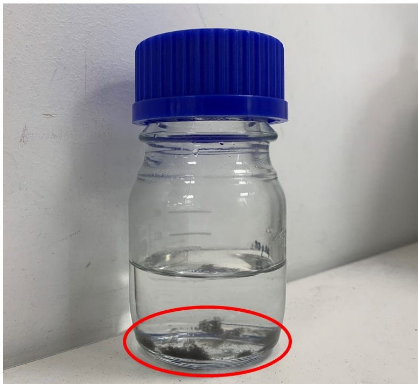
Figure 4.13: The \text{MgCl}_2 solution after prepared by dissolving the anhydrous \text{MgCl}_2 powder in distilled water
