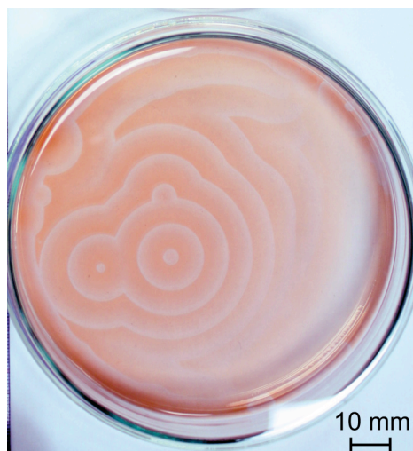
Figure 1.1 Optical image showing patterns formed by the ferroin-catalysed Belousov-Zhabotinsky reaction in a Petri dish. The blue and red regions indicate the presence of \text{Fe}^{3+} and \text{Fe}^{2+} respectively.
