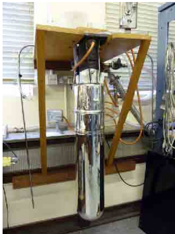
Fig. 10.2: Liquid Helium pumped glass cryostat.
