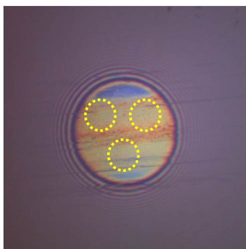
Figure 3-14 – Illustration demonstrating how specific areas of the SLIM image were selected using the SLIM film thickness software to measure the film thickness.
