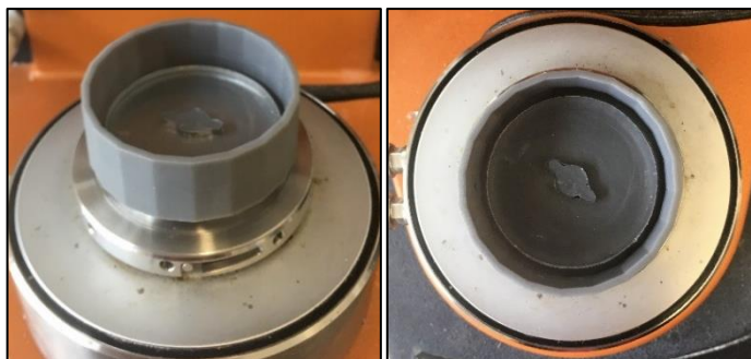
Figure 3.2 – Photographs of 3-D printed base plate (tribometer cell) for holding the PDMS disc.
