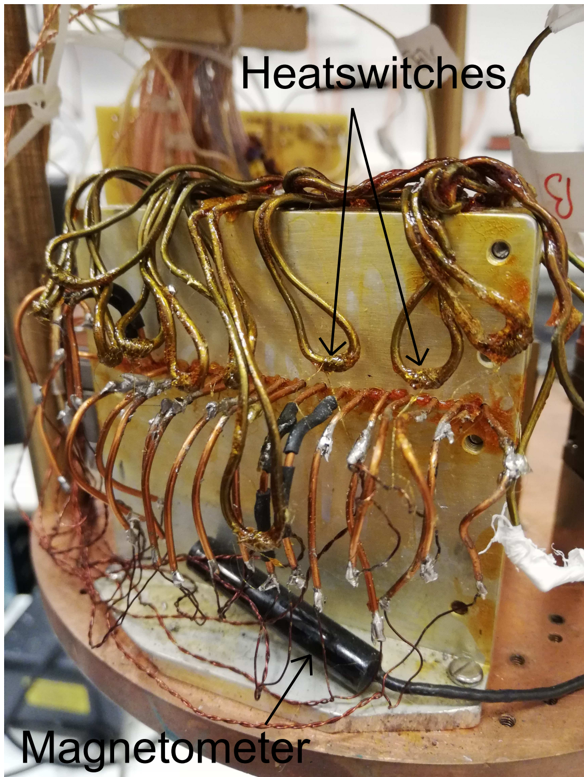
Figure 3.21: A photograph highlighting some of the heatswitches wrapped around the lead wire of the coils. The magnetometer used in the experiment is also shown.
