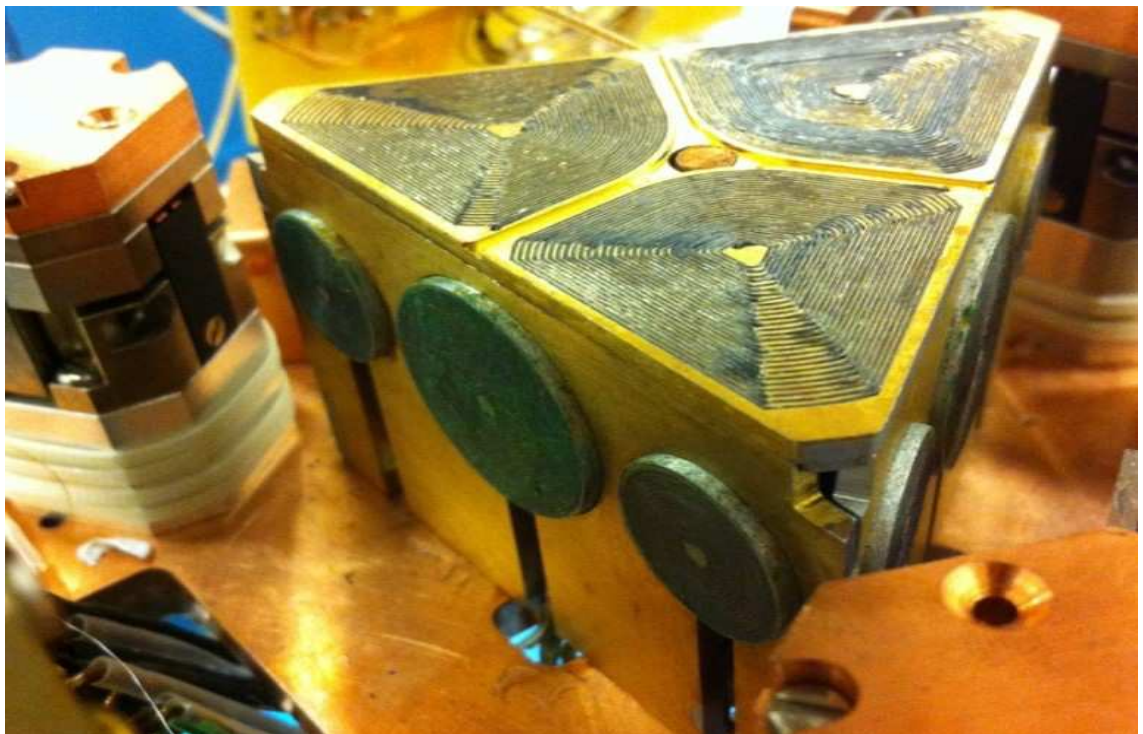
Figure 3.3: This is the bearing that held the superconducting lead coils which, through the use of persistent currents, would levitate and control the float through the Meissner effect. The photograph was taken by Collins [40].
