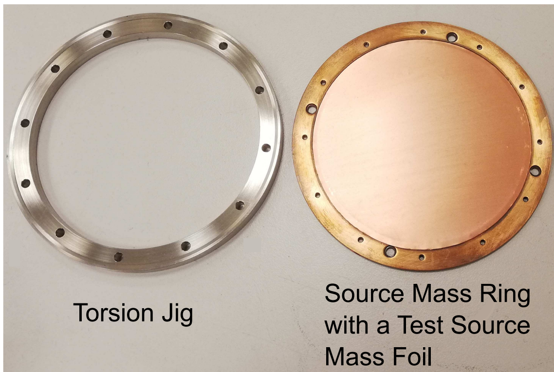
Figure 3.12: A photograph of the torsion jig and a source mass ring with a test source mass foil in place after being glued and pulled taut.
