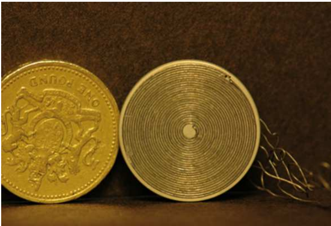
Figure 3.4: A close-up of one of the larger bearing centre side coils with a pound coin to give a sense of scale. The photograph was taken by Collins [40].
