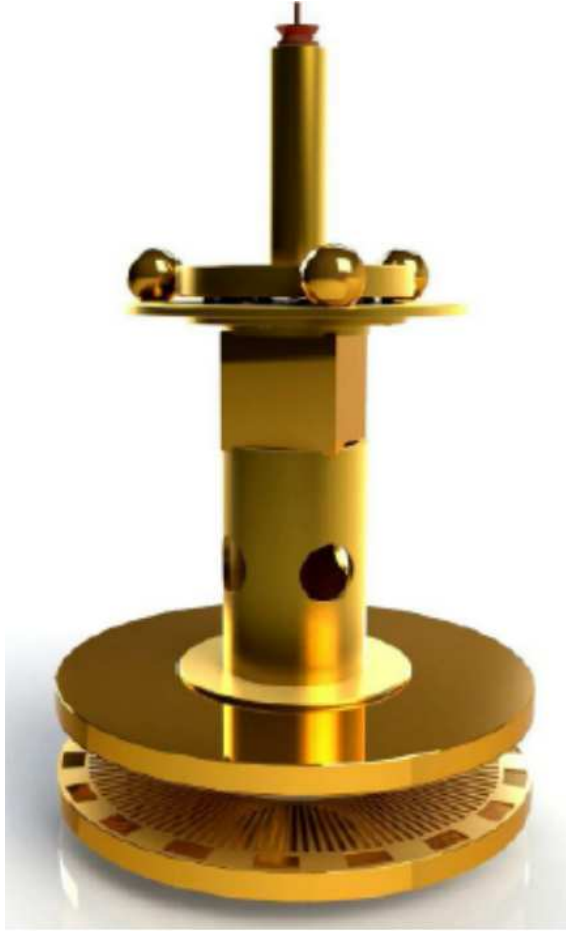
Figure 1.6: A rendering of the Eöt-Wash group's experiment's torsion balance detector and 'attractor'. The experiment was performed at the University of Washington in 2020. The render is taken from the paper by Lee et al. [25].
