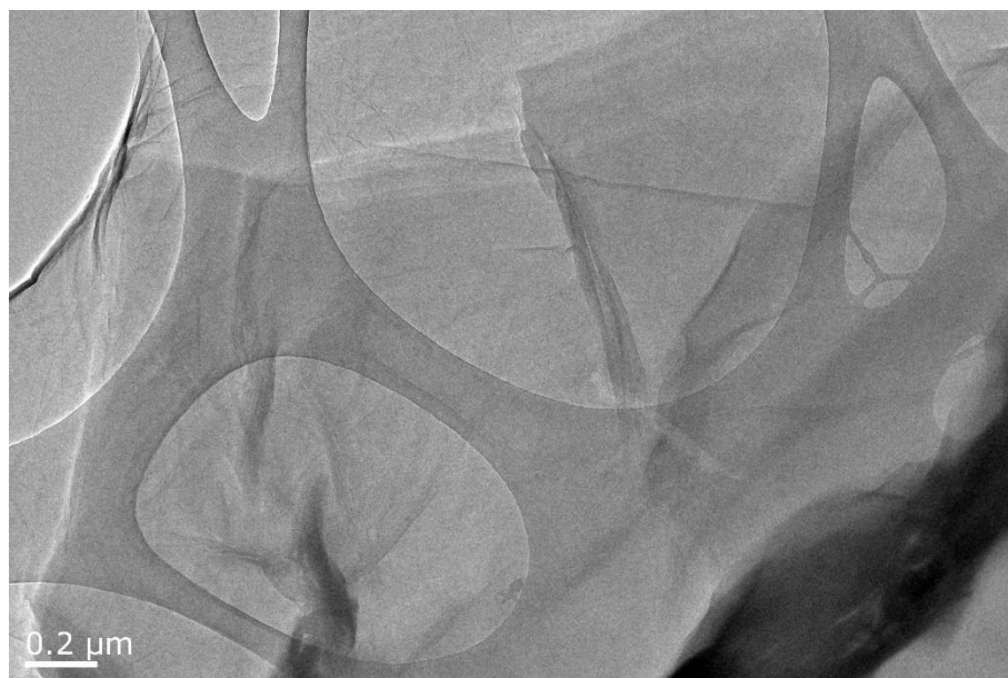
Figure 5.4 TEM image of as-prepared graphene oxide few layer sheets, with the lacey carbon TEM support film visible in the background.
