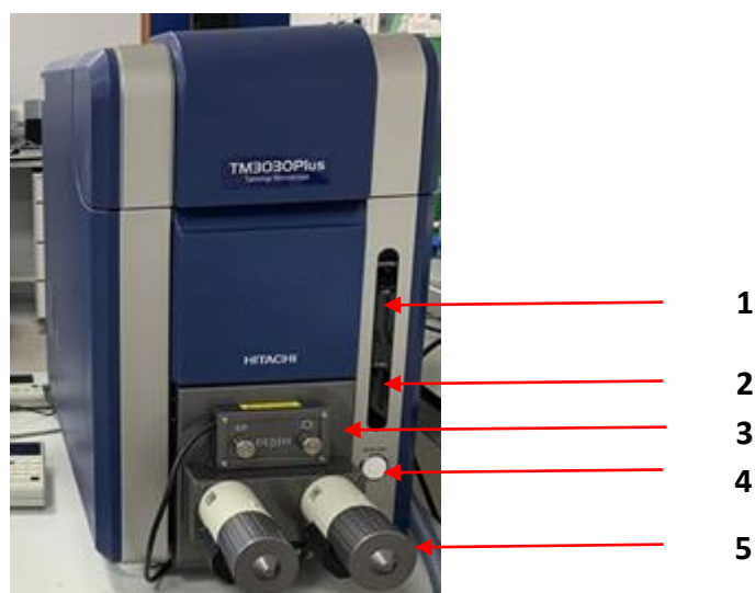
Fig. 3.2. HITACHI TM3030Plus Tabletop Scanning Electron Microscope Main Unit Front View. Components: 1- AIR mode indicator, 2- EVACUATION mode indicator, 3- Specimen Stage, 4- EVAC/AIR Switch, and 5 - X & Y axes control knobs.
