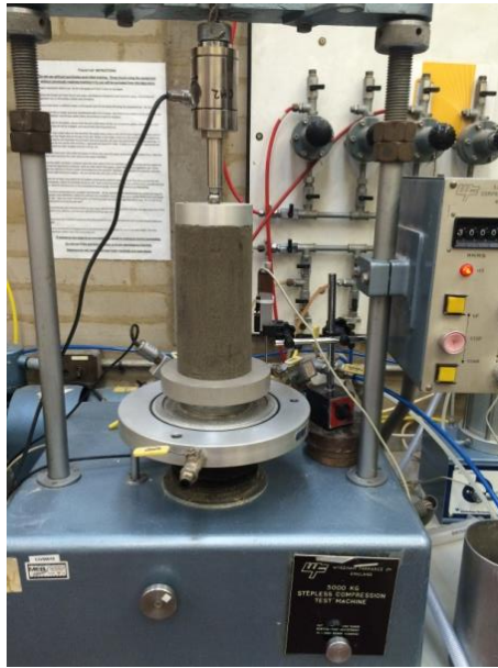
Figure 3.13 (10) kN load cell with unconfined compressive test apparatus.
