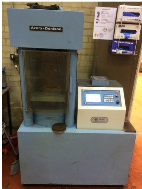
Figure 3.13 (10) kN load cell with unconfined compressive test apparatus.
