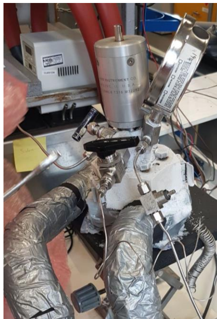
Figure 6-14 Pressure rig set-up used for CO 2 absorption testing where the lid is frozen due to the low temperature used while the hoses are insulated with foam.
