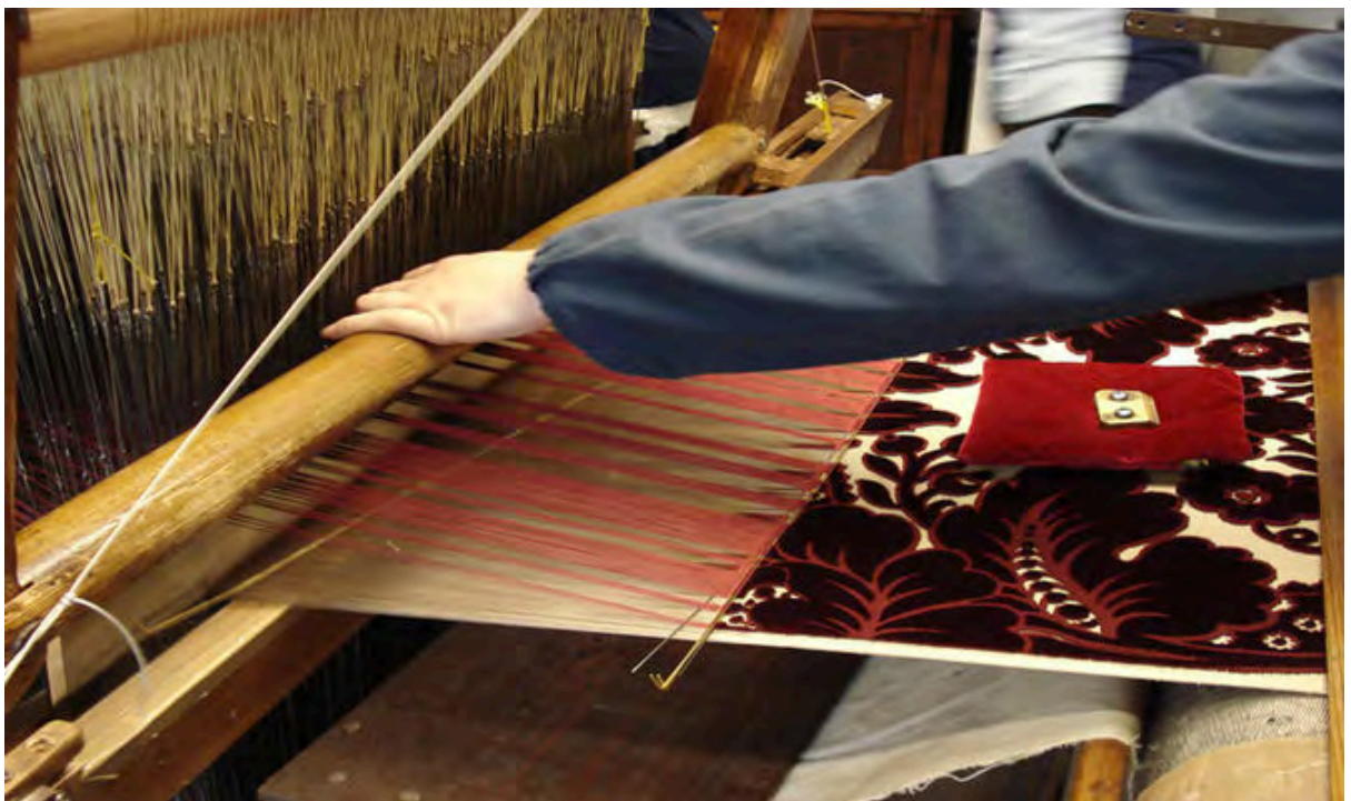
Figure 15. The precise eighteenth-century loom on which the fabric was hand-woven, pictured in the process of producing a length of cut and uncut velvet (photographer unknown).
