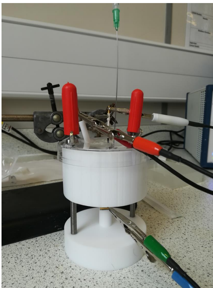
Figure 3.16 Cyclic voltammetry cell used, allowing a set diameter of the surface of the chip to be submerged (120)
