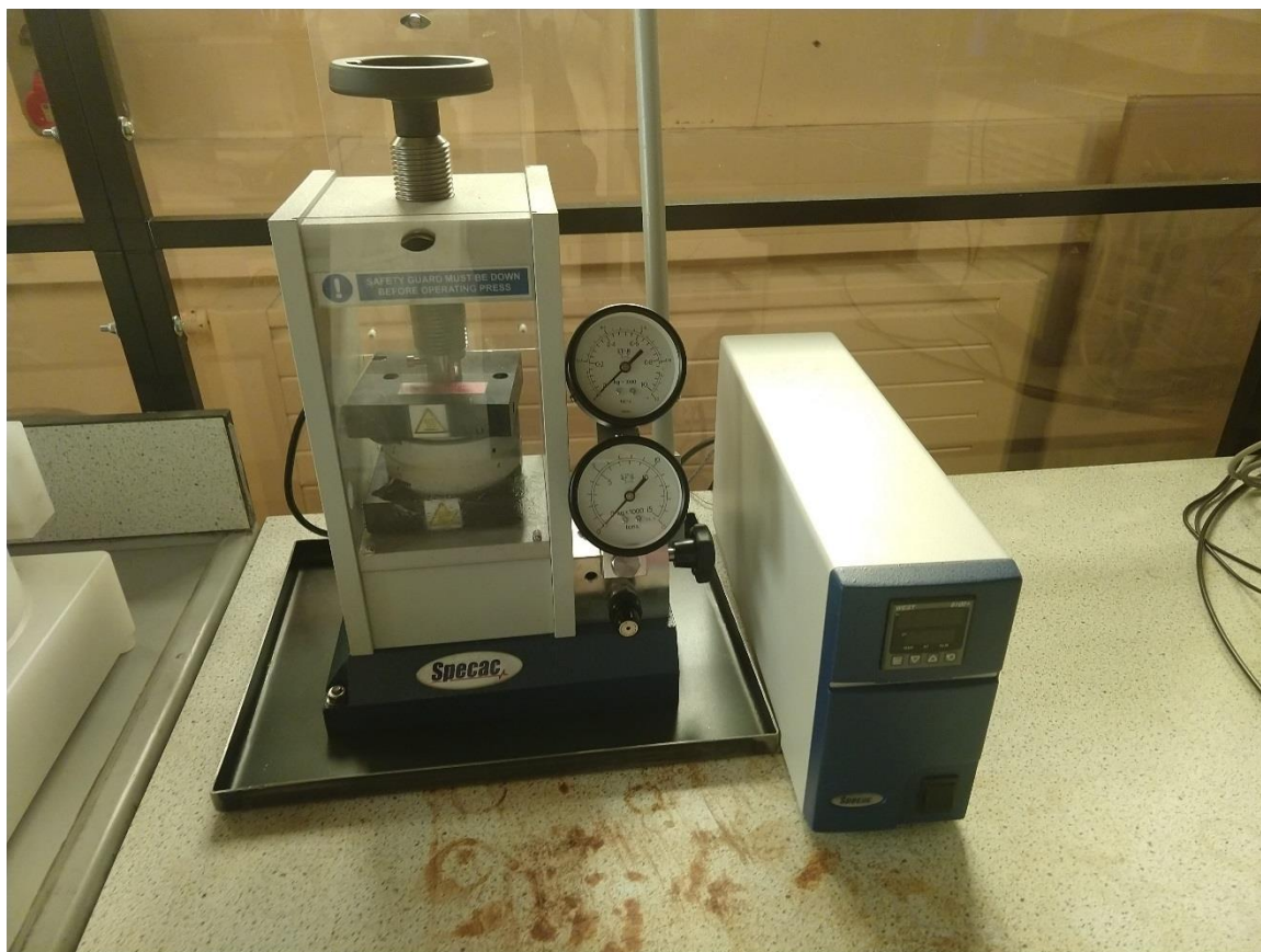
Figure 2.2 Atlas press with a heated plate used for nanoimprint lithography
