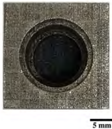
Figure 5.39 - Brazing cap produced via LPBF using heated bed and the tungsten-tantalum alloy
