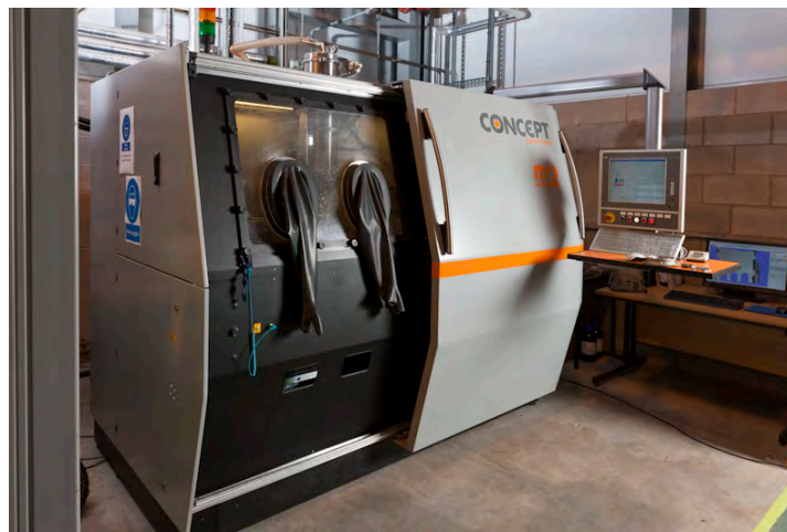
Figure A.1 - Photograph of Concept Laser M2 with powder handling chamber (left) located in M&M UoB
