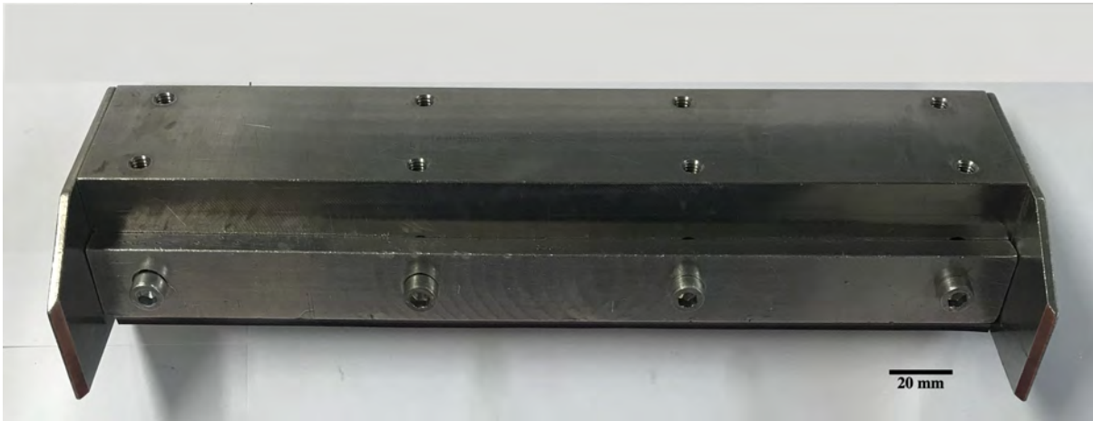
Figure A.4 - Concept Laser M2 recoater assembly
