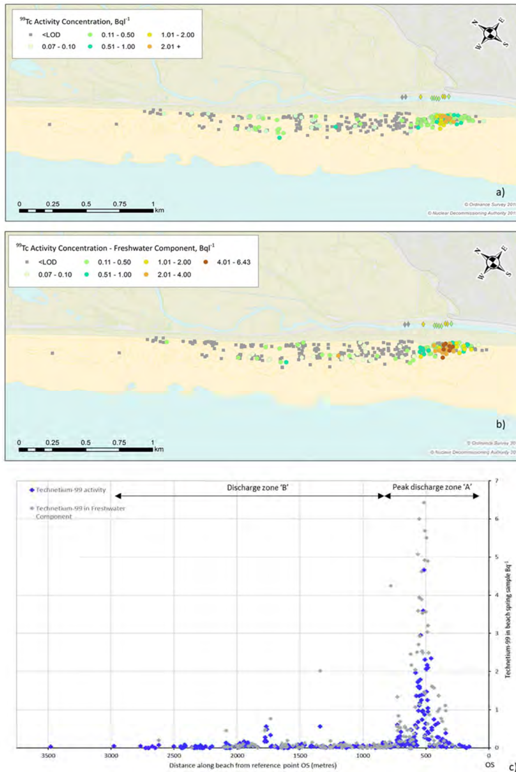
Figure 4-3 Technetium-99 plume discharge footprint 2009-2018. A distinct asymmetric plume of 2600m width, with the spring peak discharge zone area recording the highest ^{99}\text{Tc} activity levels, a) ^{99}\text{Tc} found in the spring water samples; b) calculated ^{99}\text{Tc} in spring water freshwater component; c) ^{99}\text{Tc} activity versus distance along foreshore from basepoint 'OS' (30.2267;50.2835).
