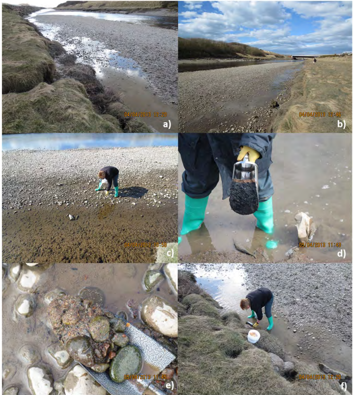
Figure 3-2 Photographs of the field visit to investigate the river-bed composition at very low water levels a) river Ehen looking south down towards the sea; b) river Ehen looking north towards the pipeline; c) consolidated gravel bed, grab samples attempted; d) example of river bank sediment grab sample; e) consolidated large gravel at the surface and subsurface, auger would not penetrate; f) sandy river bank sediment grab sample methods
