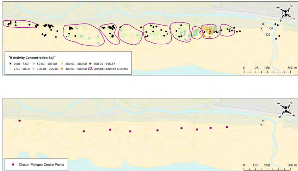
Figure 5-15 Approach to cluster samples point to single input particle exit point to represent the discharge footprint into the Sellafield groundwater model (cluster points 1-9 from N to S).
