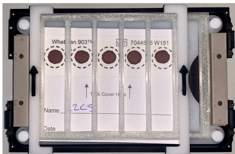
FIGURE 4.7: Picture demonstrating the use of the 3D printed template in use with a DBS collection card and LESA adapter.
