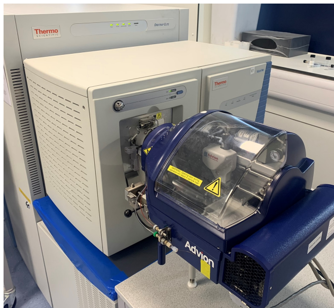
FIGURE 1.9: Image of an Advion Triversa NanoMate source coupled to an Orbitrap Elite mass spectrometer
