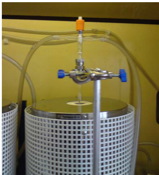
Figure 3.2 – Set-up for sample preparation in flowing inert gas.
