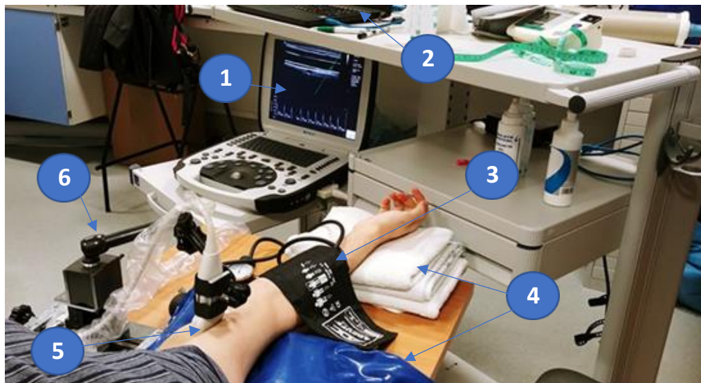
Figure 4. Full Flow Mediated Dilation (FMD) setup. Equipment shown as follows; 1) Terason Duplex Doppler Ultrasound, 2) PC laptop running CardioVascular Suite software, 3) Occlusion cuff, 4) Supports for raised arm, 5) 15-4Mhz transducer attached to Terason, and 6) Three-axes movement probe holder.
