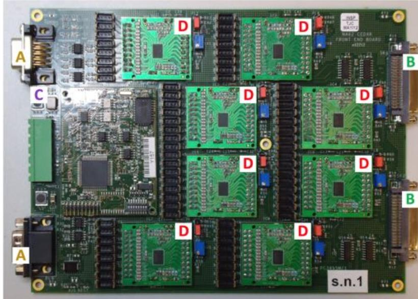
Figure 4.5: Prototype of a front-end board, with 64 analog differential inputs (indicated by the letter A), 64 differential outputs (indicated by the letter B) and an ELMB (indicated by the letter C), equipped with 8 mezzanines with 1 NINO ASIC each (indicated by the letter D).
